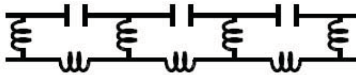
Figure 1.9: LC equivalent circuit
