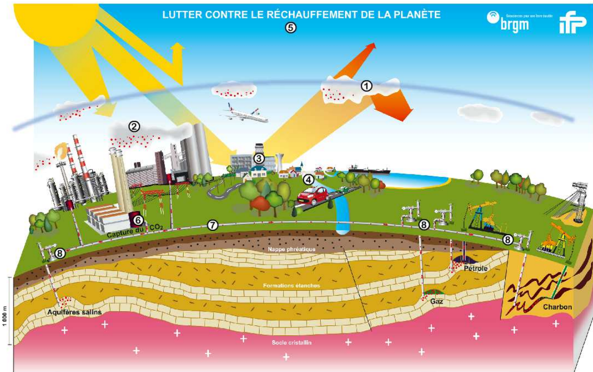
Figure 1: Carbon Capture and Storage (CCS), CO 2 is captured at electric power plants (6), transported by pipelines (7) to wells (8) where it can be injected into saline aquifers, depleted gas or oil fields or coal seams. (image source: BRGM, IFP Energies nouvelles)
