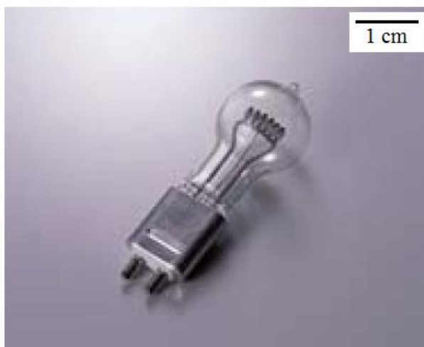
Figure 2.24: Picture of the type of lamp used for the successful growth of \text{La}_2\text{CoO}_{4+\delta} .
