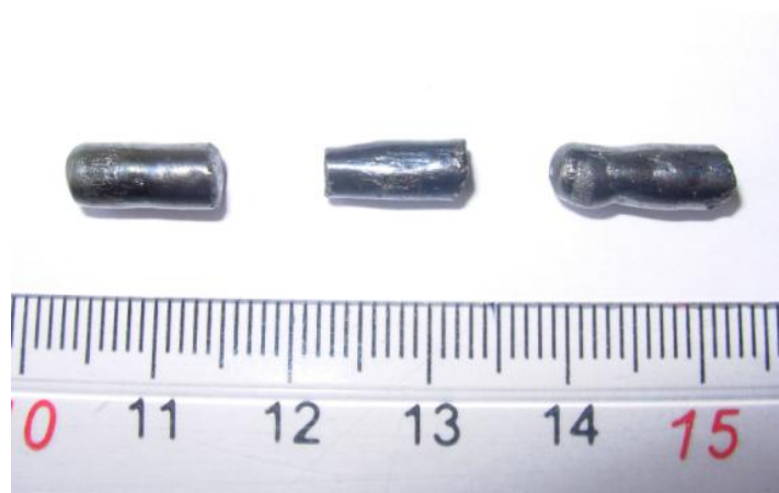
Figure 2.27: Three pieces of as grown single crystals, cut from final bulk products.
