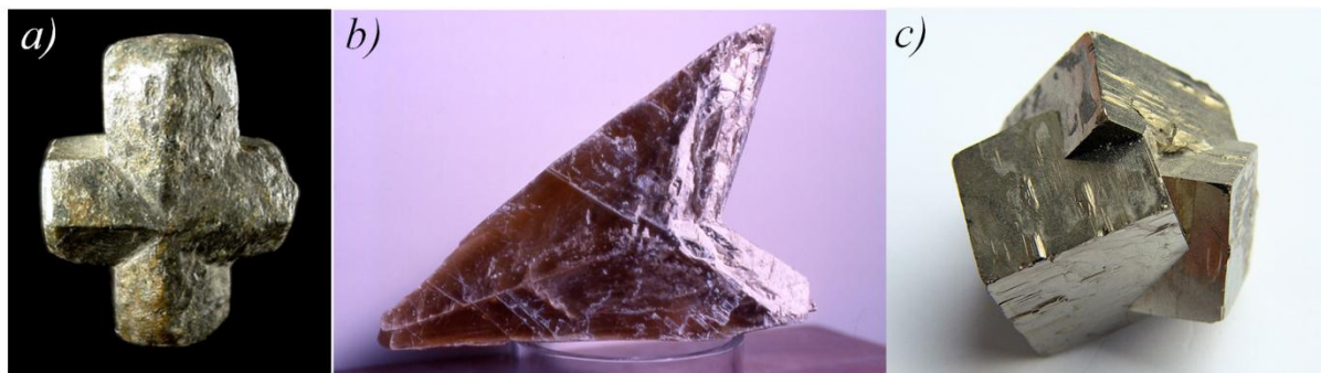
Figure 3.1: Different examples of growth twins a) Staurolite, « croix grecque », b) twinned gypsum, c) twinned pyrite.
