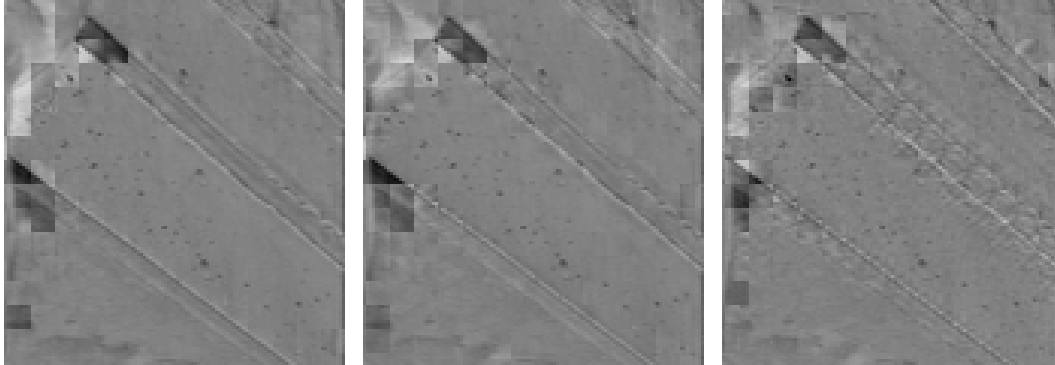
Figure 3.17: Prediction residue images of a region in Foreman using sparse prediction in comparison to ATM and NLM - (left) ATM, (middle) NLM, and (right) SP.
