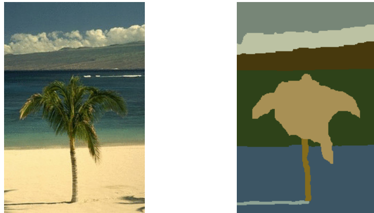
Figure 2.8: An example natural image which is composed of several textural regions - (Left) The “beach” image, and (right) the texture segmented image. Different textural regions have been shown with different colors.
