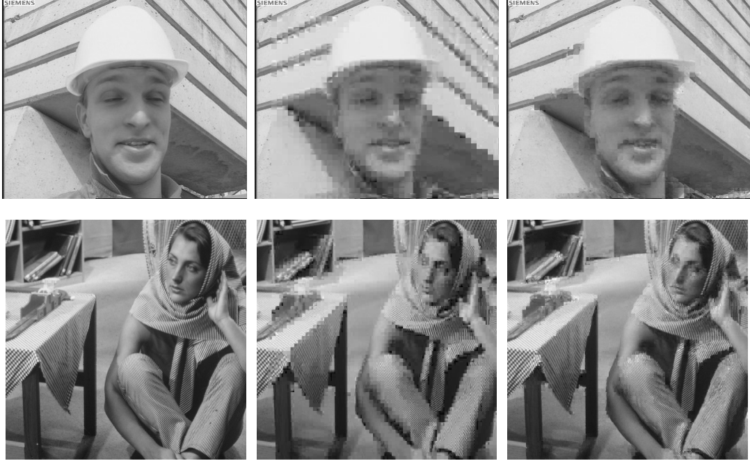
Figure 3.9: Predicted images of (top) Foreman and (bottom) Barbara using overcomplete DCT and adaptive dictionaries with dynamic approximation supports - (left) The original image, (middle) the predicted image with DCT dictionary, and (right) the predicted image with adaptive dictionaries.
