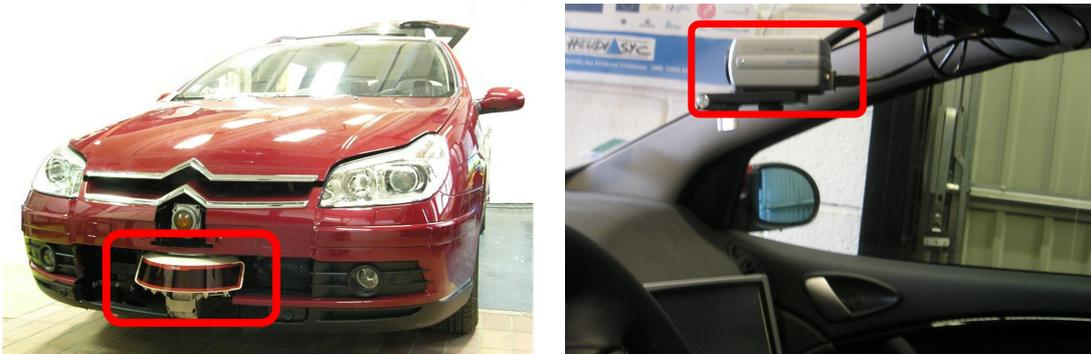
**Figure 1.18:** *Experimental platform indicating the relative locations of the sensors*
