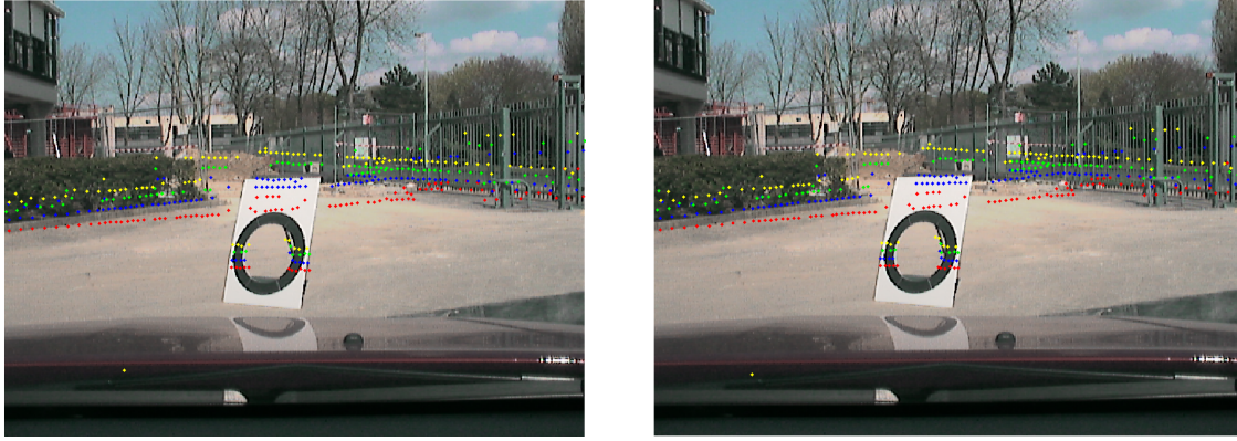
(a) Results using an unconstrained aspect ratio camera model (b) Results using a unitary aspect ratio camera model
