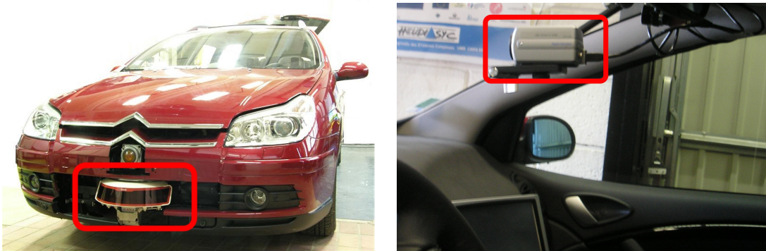
Figure 1.18: Experimental platform indicating the relative locations of the sensors
