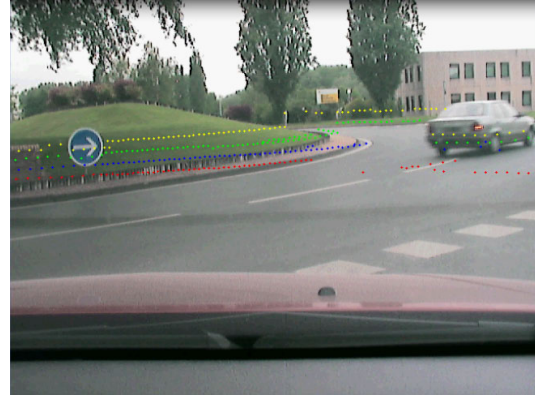
(b) Even if the camera and the lidar data is received asynchronously, their slight temporal offset is almost imperceptible in dynamic objects as observed in the figure.
