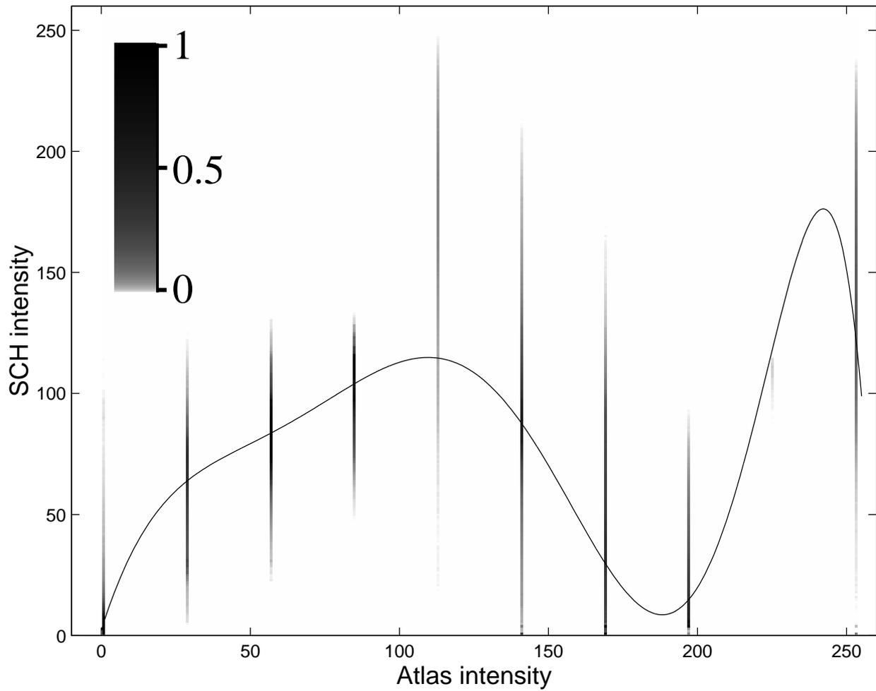
FIG. 7.8 – Intensity transformation found by registering the atlas with T1 and assuming mono-functional dependence. The function  $f$  is overlaid on the joint histogram of the two images after registration. The joint histogram values have been compressed logarithmically and normalized as is depicted in the color scale. The tissue types corresponding to the different atlas intensities are presented in table 7.1.
