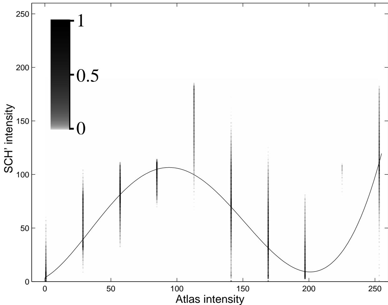
FIG. 7.12 – Intensity transformation found by registering the atlas with  $T1'$  and assuming mono-functional dependence. The function  $f$  is overlaid on the joint histogram of the two images after registration. The joint histogram values have been compressed logarithmically and normalized as is depicted in the color scale. The tissue types corresponding to the different atlas intensities are presented in table 7.1.
