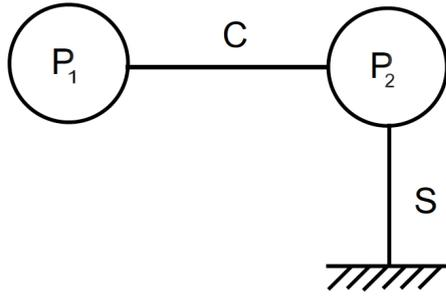
Figure 1.4: *Schematics of the differential pumping of the science cell.  $P_1$  is the MOT pressure,  $P_2$  is the pressure in the science cell,  $C$  is the conductance of the tube between the MOT chamber and the pump located at the elbow, and  $S$  is the effective pumping speed at the elbow.*
