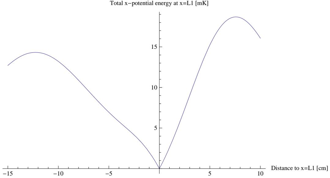
Figure 4.10: *Static trap profile in the transport direction at  $x = L_1$ . The small asymmetry is due to the coils asymmetry since  $x = L_1$  is between the MOT pair (M) and the first transport pair (T1).*
