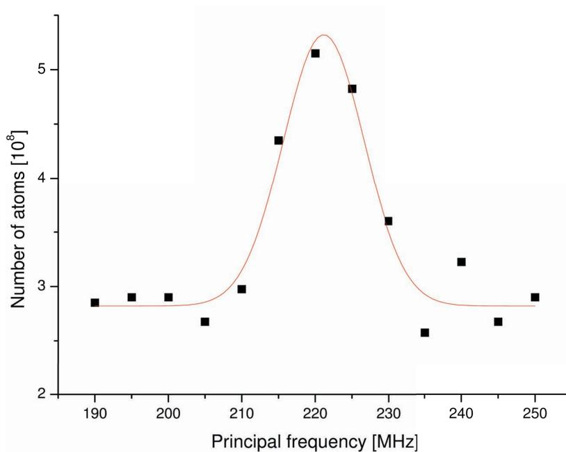
Figure 3.4: *Dependency of  $^{40}\text{K}$  atom number on the spin-polarization principal AOM frequency. The maximum corresponds to the atomic resonance. The picture has been taken after 54 ms in the magnetic trap and 2.1 ms of time-of-flight (see part 2.2.3).*
