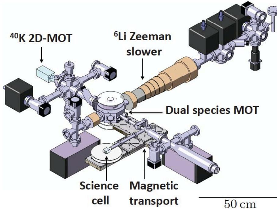
Figure 1.1: Schematics of the vacuum assembly (see also Figure 1.2). The dual-species MOT is loaded from a 2D-MOT for  $^{40}\text{K}$  and a Zeeman slower for  $^6\text{Li}$ . A magnetic transport allows to transfer the cloud to a UHV science cell with large optical access.
