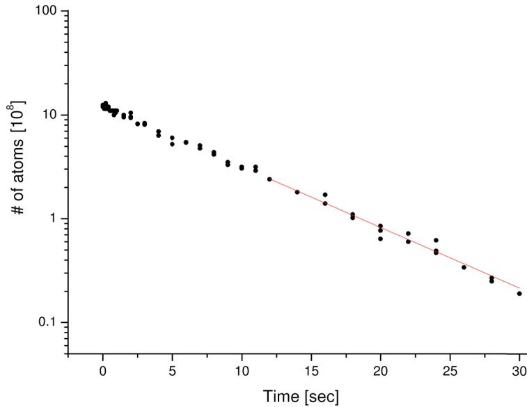
Figure 2.15: *Lifetime measurement of  $^{40}\text{K}$  MOT. At  $t = 0$ , the 2D-MOT is switched off. The long-term behavior is fitted with a single exponential decay, according to equation 2.19. The long-term decay time is found to be 7.5 s.*
