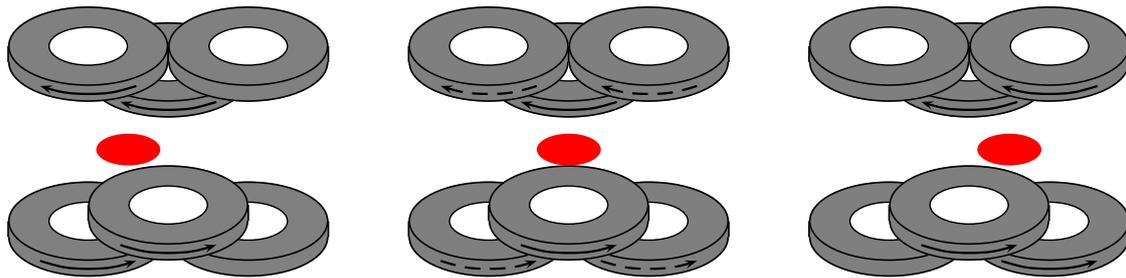
Figure 4.1: *Changing the currents in three consecutive anti-Helmholtz pairs of coils moves the center of the trap: if we decrease the current in the first pair of coils as we increase the current in the third one (see arrows), the center of the trap moves toward this third pair.*
