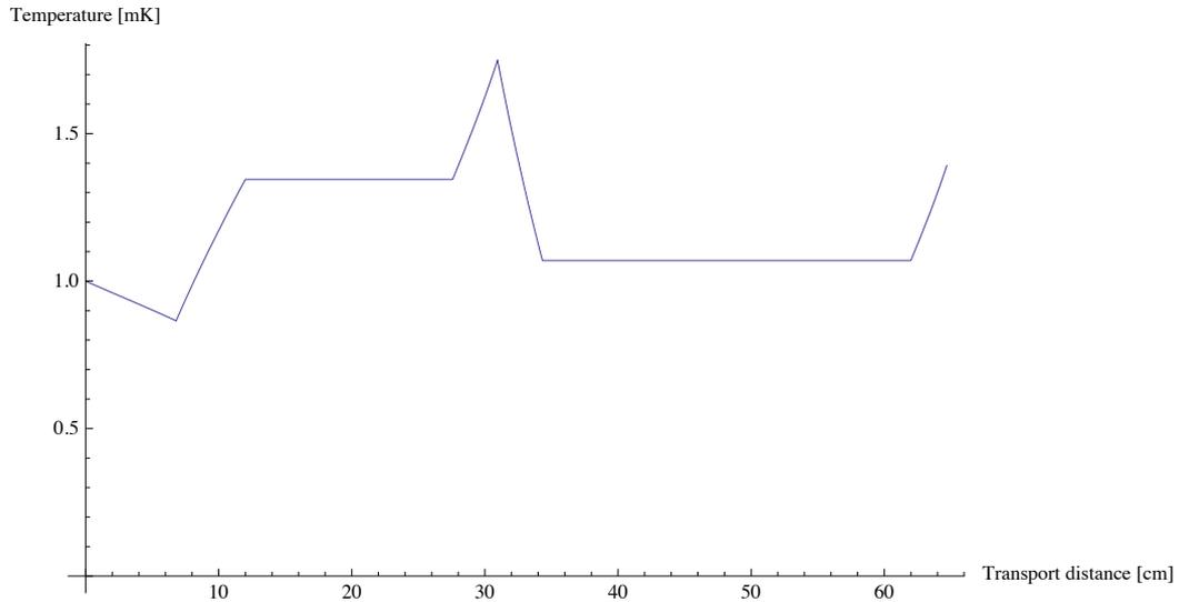
Figure 4.5: *Theoretical cloud temperature during the adiabatic transport. The initial temperature is chosen to be 1 mK. Since the cloud temperature is proportional to the initial temperature according to equation 4.7, the graph can be used for any initial temperature by adding the initial factor.*
