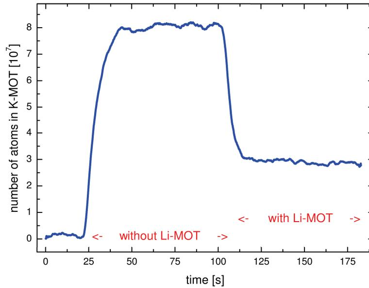
Figure 2.16:  $^{40}\text{K}$ -MOT number of atoms in presence or not of  $^6\text{Li}$ -MOT. The loading rate of  $^{40}\text{K}$  is reduced in order to have a small  $^{40}\text{K}$ -MOT and a constant  $^6\text{Li}$  density. The axial gradient magnetic gradient is increased to  $16\text{ G.cm}^{-1}$  in order to increase the densities and thus the inelastic losses.
