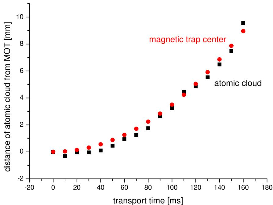
Figure 5.3: Position of the  $^{40}\text{K}$  cloud and the theoretical trap center as a function of transport time, for a constant acceleration of  $0.7 \text{ m}\cdot\text{s}^{-2}$ . The cloud position is obtained by absorption imaging (see part 2.2.2).
