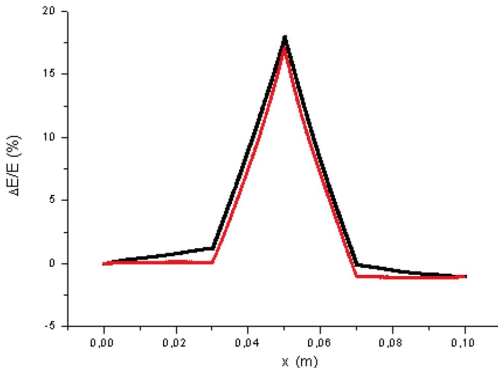
Figure 4.20: Numerically simulated relative variation of energy for 10000  $^{40}\text{K}$  atoms (black) and 10000  $^6\text{Li}$  atoms (red), due to a local magnetic defect in the sequence. The defect is 4 cm long and corresponds to a relative variation of 50 % on the gradients. The simulation has been performed in Fortran 90, using a fourth order Runge-Kutta routine [140].
