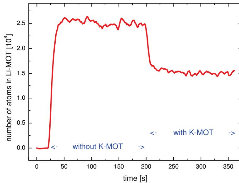
Figure 2.17:  $^6\text{Li}$ -MOT number of atoms in presence or not of  $^{40}\text{K}$ -MOT. The loading rate of  $^6\text{Li}$  is reduced in order to have a small  $^6\text{Li}$ -MOT and a constant  $^{40}\text{K}$  density. The axial gradient magnetic gradient is increased to  $16\text{ G.cm}^{-1}$  in order to increase the densities and thus the inelastic losses.
