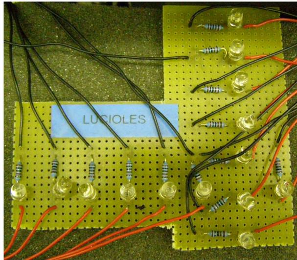
Figure 4.27: *In parallel with each coil a LED is placed in series with a  $1\text{ k}\Omega$  resistance, in order to control where the current is flowing.*
