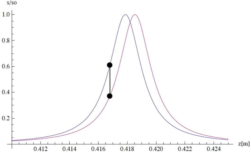
Figure 1.14: Evolution of the normalized saturation parameter with distance for a speed  $v_c/2$  (blue) and  $v_c/2 - 1 \text{ m.s}^{-1}$  (pink). In the operating regime (blue), an atom experiencing an unexpected deceleration (pink) will be less resonant and thus will be less decelerated by the slower. Therefore, it will move forward until it reaches the good  $s/s_0$  value and stick back to the operating regime downstream.
