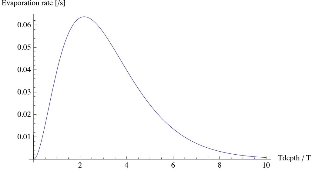
Figure 5.15:  $^{40}\text{K}$  evaporation rate in the transported magnetic trap as a function of the evaporation parameter  $\eta = T_{\text{depth}}/T$  (see equation 5.5). The evaporation rate is defined as the rate of atoms that reach an energy higher than the trap depth after an elastic collision.
