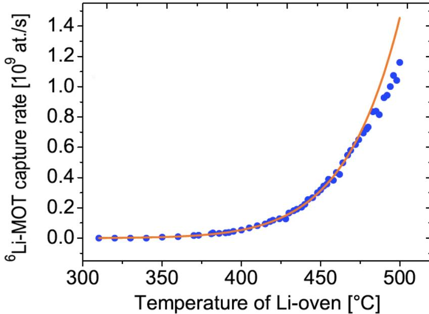
Figure 1.16:  ${}^6\text{Li}$  MOT loading rate as a function of oven temperature. The solid curve is a fit using the theoretical flux of the Zeeman slower (see equations 1.18 and 1.21). The fit is good until  $475^\circ\text{C}$ , where it starts to diverge from the experimental data, showing that our ballistic model is not valid anymore: intrabeam collisions inside the collimation tube and collisions with MOT atoms occur.
