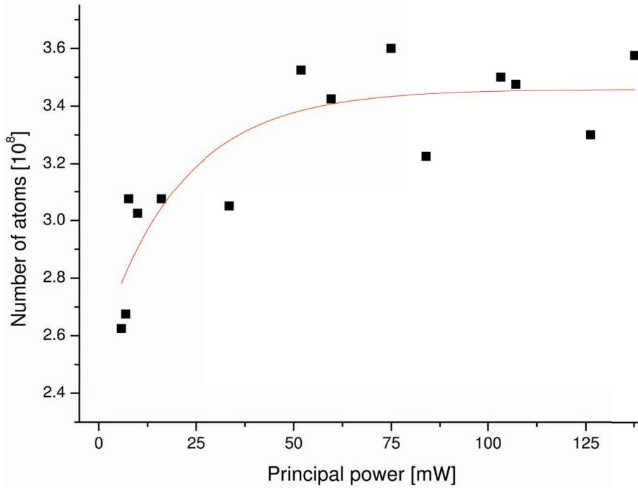
Figure 3.5: *Dependency of the  $^{40}\text{K}$  atom number on the power of the spin-polarization principal beam. As far as it is concerned, repumping power equals 30 mW. The picture has been taken after 54 ms in the magnetic trap and 2.1 ms of time-of-flight (see part 2.2.3).*
