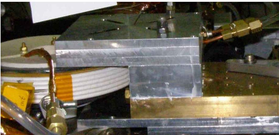
Figure 4.24: *Pulling coil ( $T1/2$ ) placed in between the MOT pair ( $M$ ) and the first transport pair ( $T1$ ). In addition, a fifth single one is placed on top in order to generate a small bias field, if necessary during injection. See engineering drawings in appendix A.6.*
