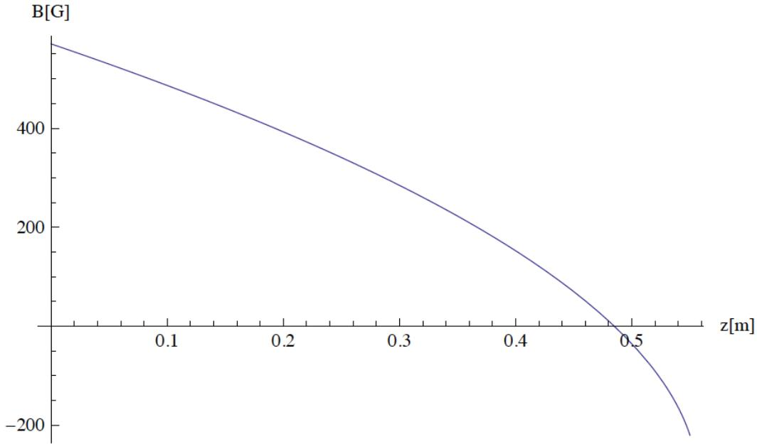
Figure 1.13: *Ideal magnetic profile of the  ${}^6\text{Li}$  Zeeman slower, plotted from equation 1.8 with  $v_c = 838 \text{ m.s}^{-1}$ ,  $l = 55 \text{ cm}$ ,  $\delta = -75 \Gamma$  and  $\alpha = 0.34$ .*
