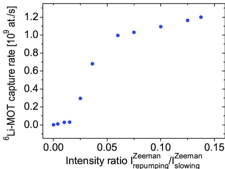
Figure 1.21:  ${}^6\text{Li}$  capture rate as a function of the ratio between Zeeman repumping and slowing intensities. The slowing power is kept to 45 mW. We see that without repumping the efficiency of the slower is very small, which we attribute to the zero field depolarizing region of the spin-flip slower. On the other hand, we only need a few milliwatts of repumper light since the efficiency saturates quickly.
