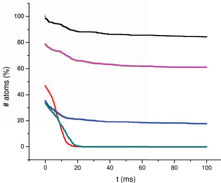
Figure 5.9: Numerical simulation of the percentage of  $^{40}\text{K}$  atoms remaining in a static quadrupole trap with  $b_y = -100 \text{ G.cm}^{-1}$  as a function of time, for various conditions:  $T = 0.5 \text{ mK}$  and DN10 tube (black),  $T = 1 \text{ mK}$  and DN16 tube (pink),  $T = 1 \text{ mK}$  and DN10 tube (blue),  $T = 0.5 \text{ mK}$  and DN10 tube misaligned by 5 mm (red),  $T = 1 \text{ mK}$  and DN10 tube misaligned by 5 mm (green).
