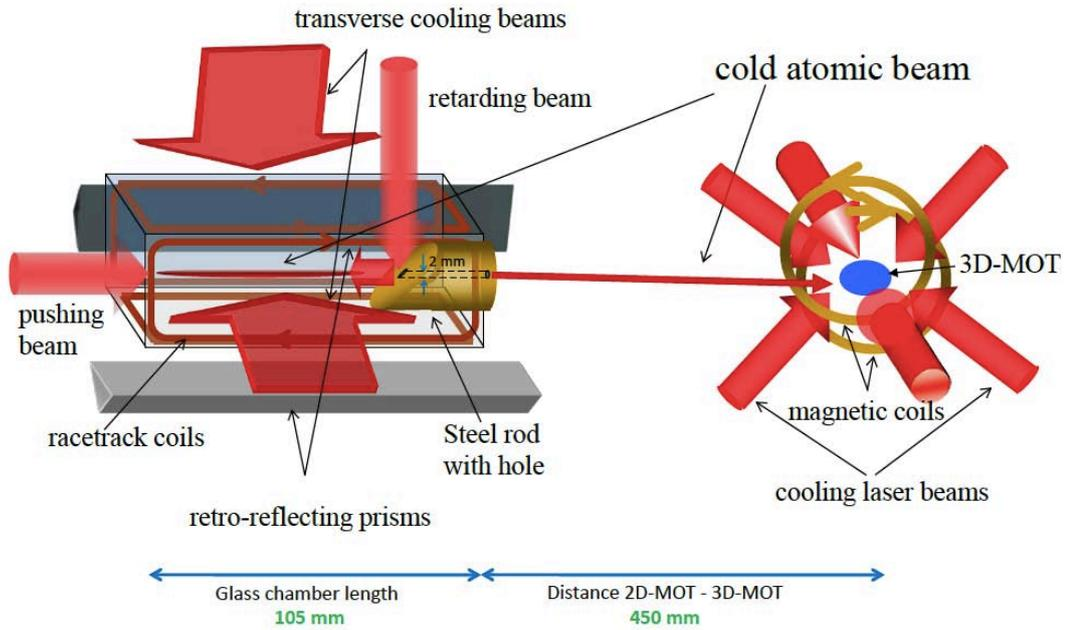
Figure 1.22: Scheme of the  $^{40}\text{K}$  2D-MOT loading of the MOT.
