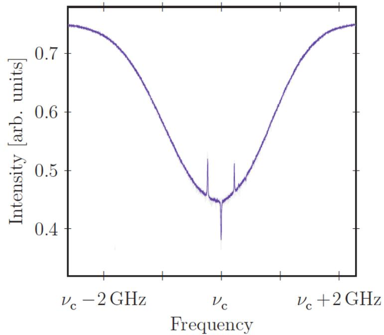
Figure 3.15: *Saturated absorption lines of the  $4S_{1/2}-5P_{3/2}$  transition of  $^{39}\text{K}$ . The middle peak is the crossover between the two others peaks that correspond to the transitions from the two hyperfine ground-states to the upper unresolved multiplet.*
