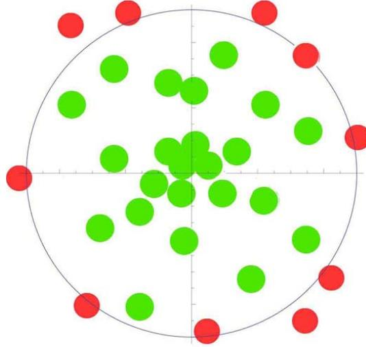
Figure 5.8: *Cartoon of the analytical (see equation 5.2) and numerical models for the truncation of the atomic distribution: each time an atom have enough energy to reach the walls of the differential pumping tube, it is lost (red).*
