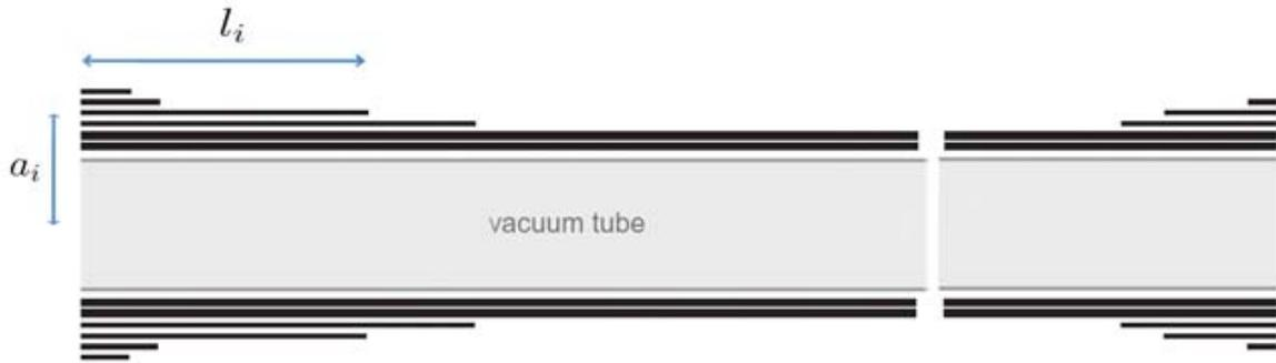
Figure 1.17: *Sectional drawing of the numerical model of the  ${}^6\text{Li}$  Zeeman slower. Each side of the spin-flip Zeeman slower is made from superimposed solenoids of length  $l_i$  and radius  $a_i$  ( $i = 1, N$ ).*
