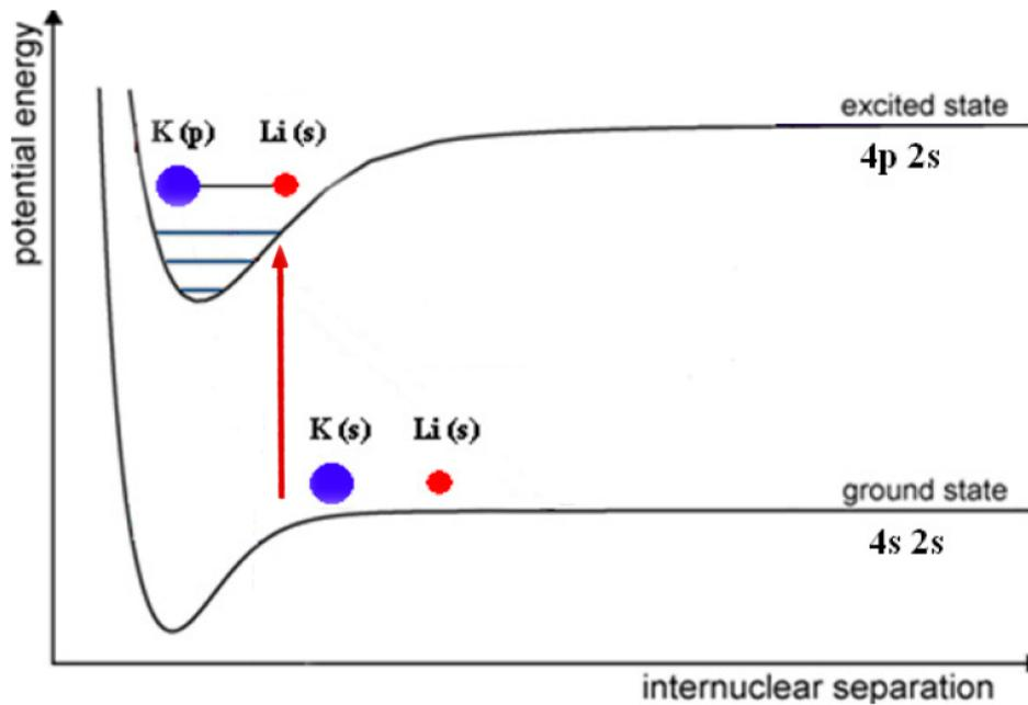
Figure 2.18: Principle of  ${}^6\text{Li}{}^{40}\text{K}^*$  photoassociation. A laser beam, red-detuned with respect to a  ${}^{40}\text{K}$  atomic asymptotic transition, is resonant with a transition towards a rovibrational bound-state of one of the excited electronic states of the molecule.
