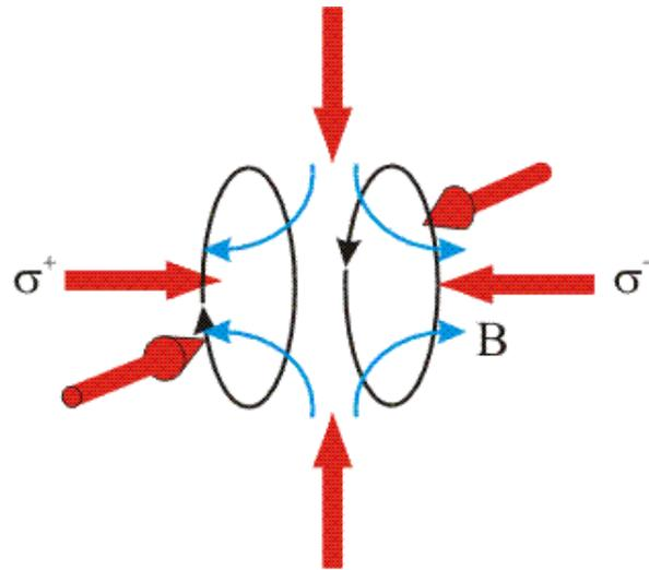
Figure 2.3: Schematics of a magneto-optical trap. In addition to quadrupolar magnetic trapping (field lines in blue), generated by a pair of anti-Helmholtz coils (see part 3.1.1), a radiative cooling is realized through two counter-propagating laser beams per direction of space (red). Those two beams have opposite circular polarizations with respect to the chosen quantification axis.
