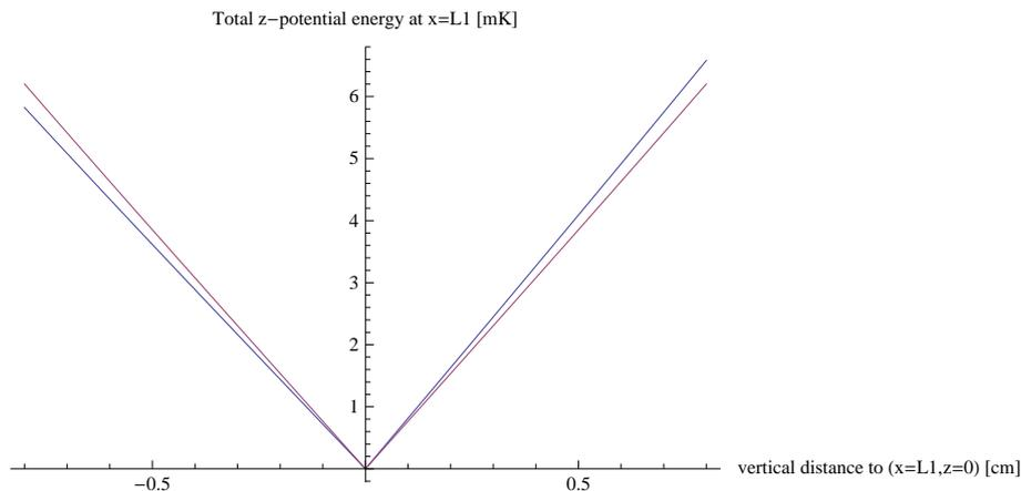
Figure 4.21: Vertical trap profile at  $x = L_1$ , with (blue) and without (pink) the gravitational tilt. There the vacuum tube has a DN16 size (0.8 cm radius), and the position  $x = L_1$  is 9 mm away from the DN10 transport tube (0.5 cm radius).
