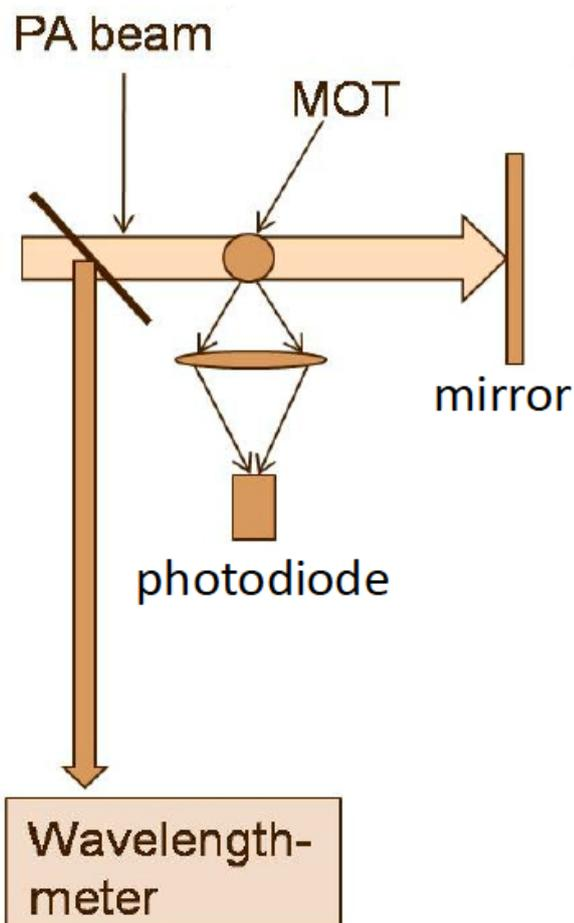
Figure 2.19: *Experimental setup of the photoassociation experiment. The photoassociation laser is sent to the MOT. While its frequency is swept, the numbers of atoms in the MOT are recorded through fluorescence (see part 2.2.1). A diminution of the number of atoms is a signature of photoassociation process, according to equation 2.22.*
