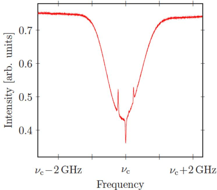
Figure 1.9: Saturated absorption  $D2$  lines of  $^{39}\text{K}$  (see appendix A.1 for the  $^{39}\text{K}$  hyperfine spectrum). The middle peak is the crossover peak used for lock. The two others correspond to the transitions from the two hyperfine ground-states to the upper unresolved multiplet (see Figure 1.6).
