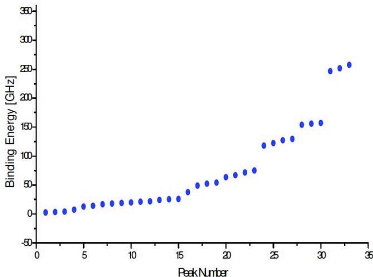
Figure 2.22:  ${}^6\text{Li}^{40}\text{K}^*$  photoassociation binding energies by increasing order.
