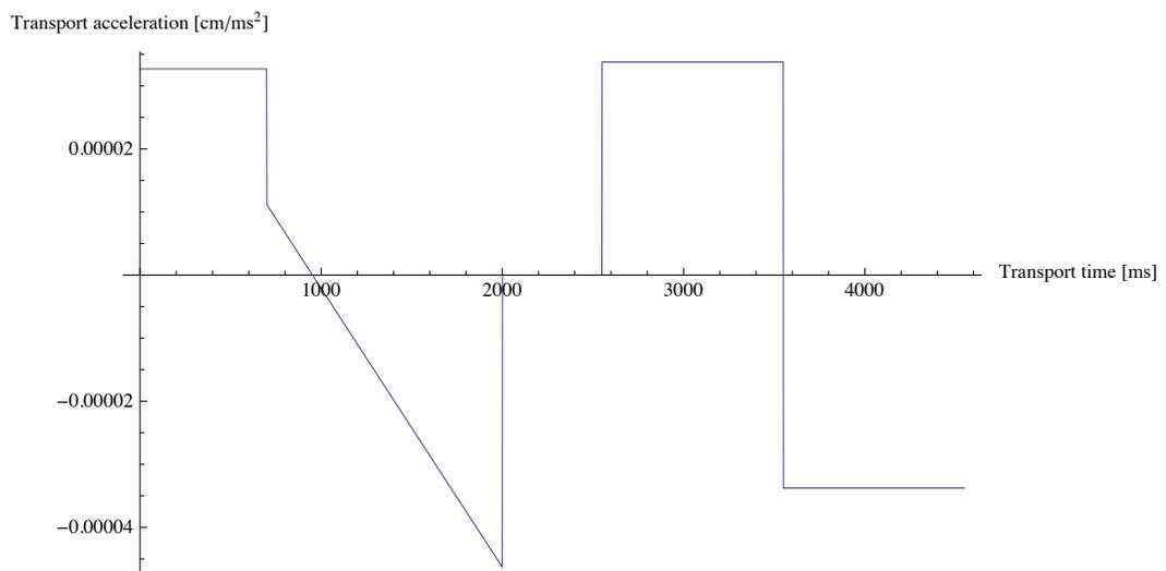
Figure 4.14: *Acceleration of the center of the trap.*
