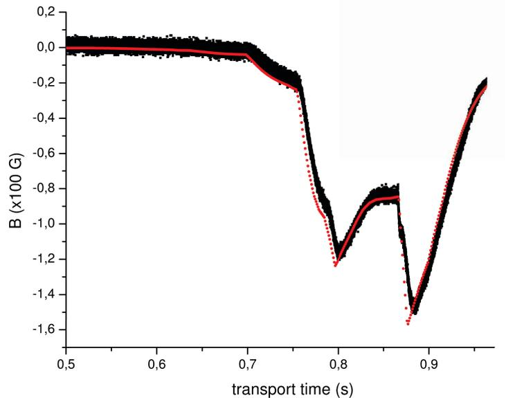
Figure 5.1: *Measurement (black) of the  $x$ -field at the center of the final quadrupole pair as a function of the transport time. Theoretical calculation (red) obtained with the transport program. The total transport sequence lasts 1 s here. The measurement was performed before assembling the transport system on the experiment, with a homemade Hall probe mounted on a  $xyz$ -translation mount.*
