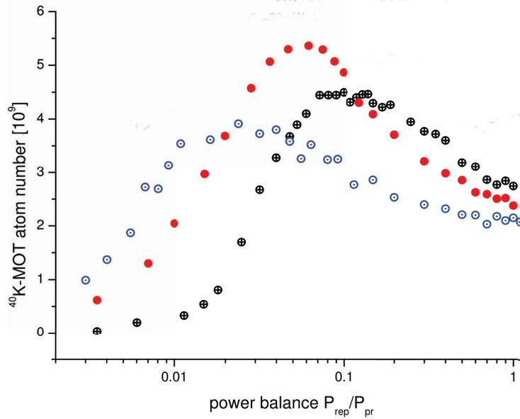
Figure 2.11: Number of atoms in single  $^{40}\text{K}$ -MOT as a function of the ratio between repumping and cooling powers, for different detunings of the repumper frequency:  $-3\ \Gamma$  (black, cross),  $-5\ \Gamma$  (red, full) and  $-7\ \Gamma$  (blue, point). The cooling power is kept at  $40\ \text{mW}$  in each beam.
