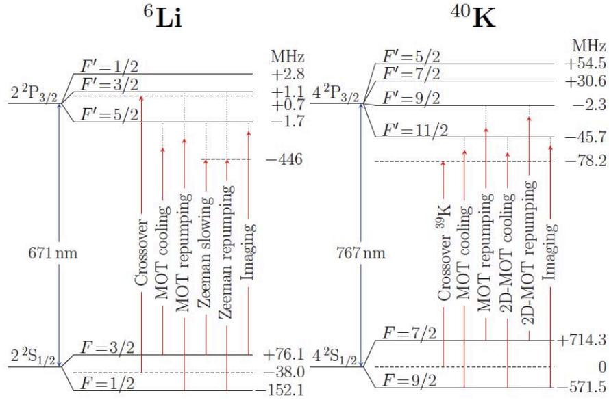
Figure 1.6: *Hyperfine structures of  ${}^6\text{Li}$  and  ${}^{40}\text{K}$  D2 lines. The laser diodes are locked to the indicated crossover frequencies. For potassium, due to the low natural abundance of  ${}^{40}\text{K}$ , the lock is performed on a  ${}^{39}\text{K}$  crossover line (see appendix A.1 for the  ${}^{39}\text{K}$  hyperfine spectrum).*
