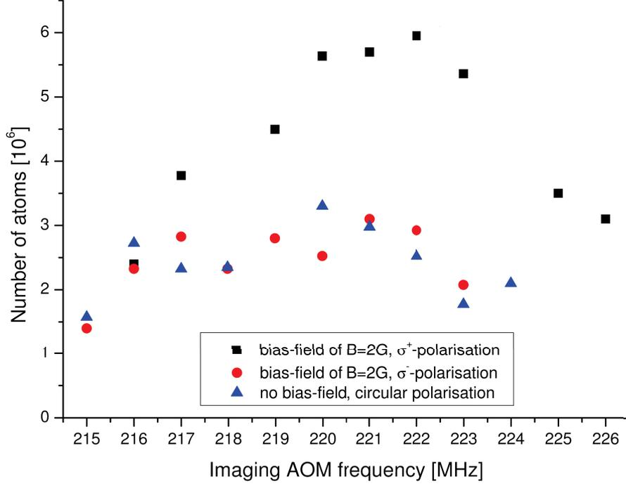
Figure 2.6:  $^{40}\text{K}$  Number of atoms in the science cell after 1.1 ms time-of-flight as a function of imaging frequency, for different imaging configurations. The bias field is vertical and parallel to the imaging beam.
