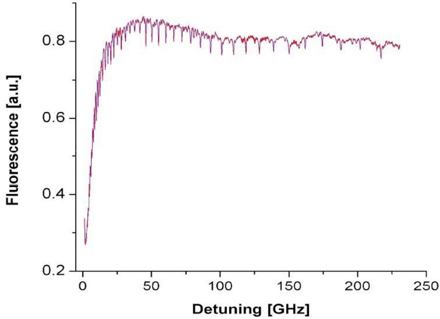
Figure 2.20: Fluorescence of single  $^{40}\text{K}$  MOT as a function of the photoassociation detuning ( $-\delta$ ) with respect to the cooling transition. Note that close from resonance the photoassociation beam is harmful for the MOT, as expected. Note also that the atom density is maximal at intermediate detunings due to the attractive optical dipole forces (see part 3.4.4) created by the intense photoassociation beam. The experimental setup is described in Figure 2.19.
