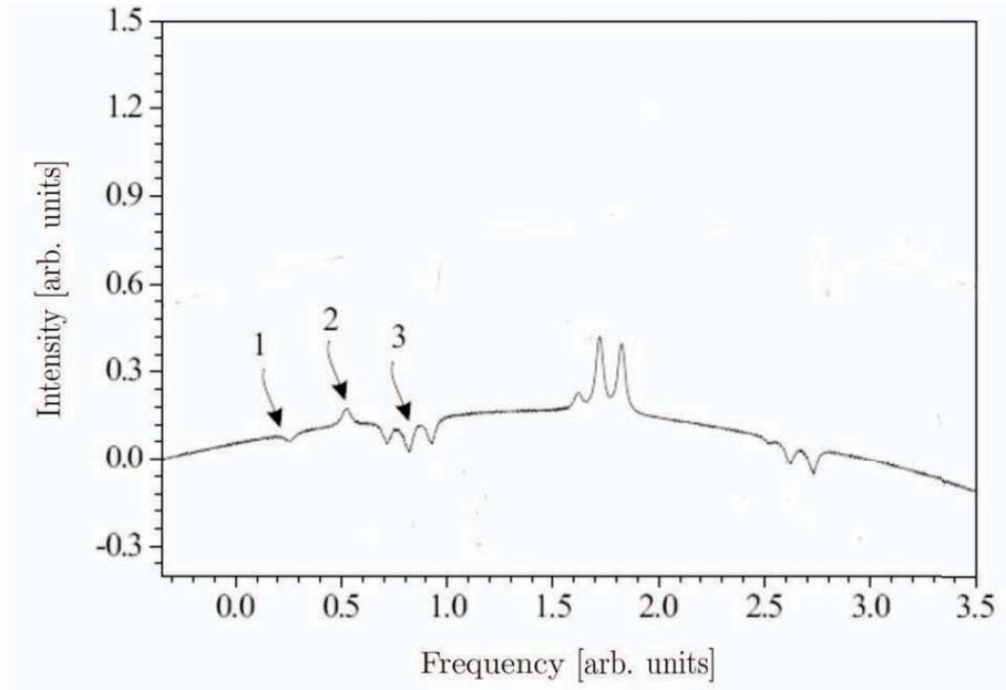
Figure 1.8: Saturated absorption D2 lines of  ${}^6\text{Li}$ . Peak 2 is the crossover peak used for lock. Peaks 1 and 3 correspond to transitions from the two hyperfine ground-states to the upper unresolved multiplet (see Figure 1.6). The unmarked peaks are the D1 lines of  ${}^7\text{Li}$ .
