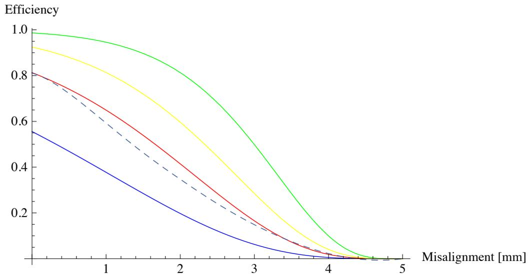
Figure 5.12: *Theoretical efficiency of trapping  ${}^6\text{Li}$  and  ${}^{40}\text{K}$  atoms in a static magnetic trap of gradient  $93\text{ G.cm}^{-1}$  in a DN10 tube as a function of misalignment, for four temperatures:  $0.3\text{ mK}$  (green),  $0.4\text{ mK}$  (yellow),  $0.5\text{ mK}$  (red), and  $0.7\text{ mK}$  (blue). The model used is given in equations 5.2 and 5.4. In addition, a numerical simulation at  $0.5\text{ mK}$  in an identical magnetic trap is shown (dashed line).*
