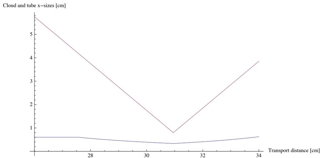
Figure 4.8: *Theoretical RMS size (see equation 4.4) of the transported cloud (blue), and radius of the tube (pink) along  $x$ . Zoom around the elbow. To define the tube size in the transport direction we have taken the minimal distance to the walls.*
