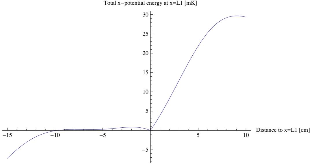
Figure 4.11: *Dynamical trap profile in the transport direction at  $x = L_1$ , including a critical inertia tilt of  $a_{max}^* = 28 \text{ m.s}^{-2}$ . Due to non-linearities, the dynamical capture region in the transport axis is reduced to approximately 2 cm.*
