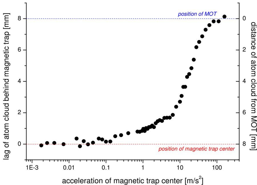
Figure 5.4: Lag of  $^{40}\text{K}$  cloud with respect to a theoretical trap center position (8 mm) as a function of the trap acceleration.
