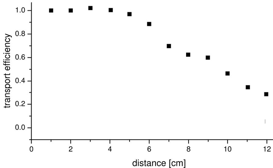
Figure 5.7: *Initial transport efficiency of  $^{40}\text{K}$  as a function of transport distance. Each point is an average over 6 measurements. The efficiency at a given point is defined as the ratio between the number of atoms measured after a round-trip to this point and the number of atoms in a fixed magnetic trap during the same duration. The initial number is  $5 \times 10^8$  in the magnetic trap.*
