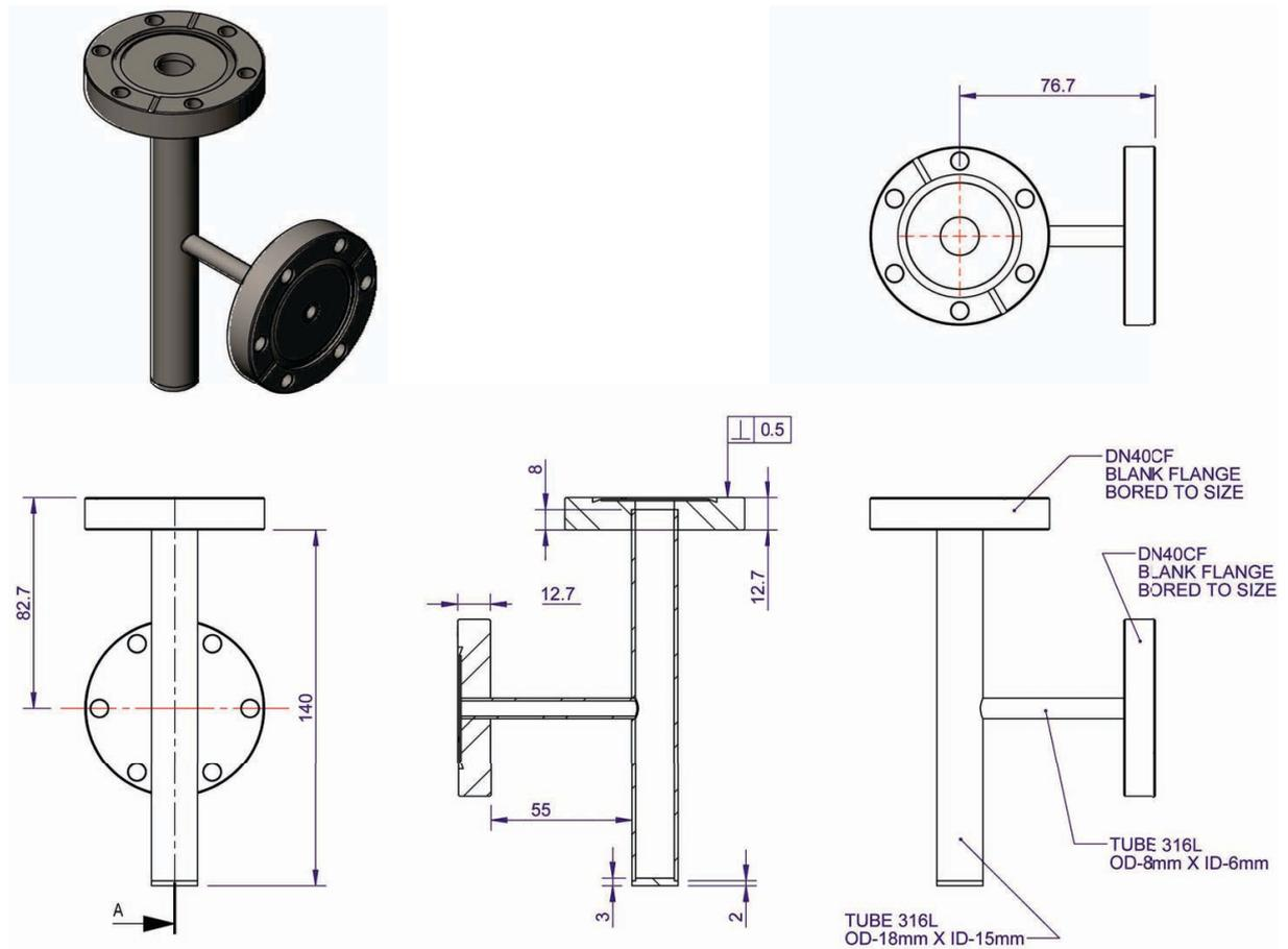
Figure A.3:  ${}^6\text{Li}$  oven (dimensions in millimeters).
