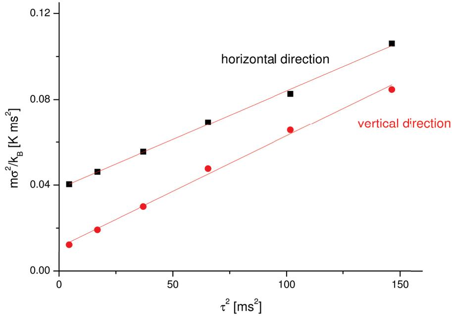
Figure 5.5: *Time-of-flight (see part 2.2.3) of the  $^{40}\text{K}$  cloud after a transport round-trip to 1 cm in 200 ms. The linear fits give a vertical temperature of  $517\ \mu\text{K}$  and an horizontal one of  $455\ \mu\text{K}$ .*
