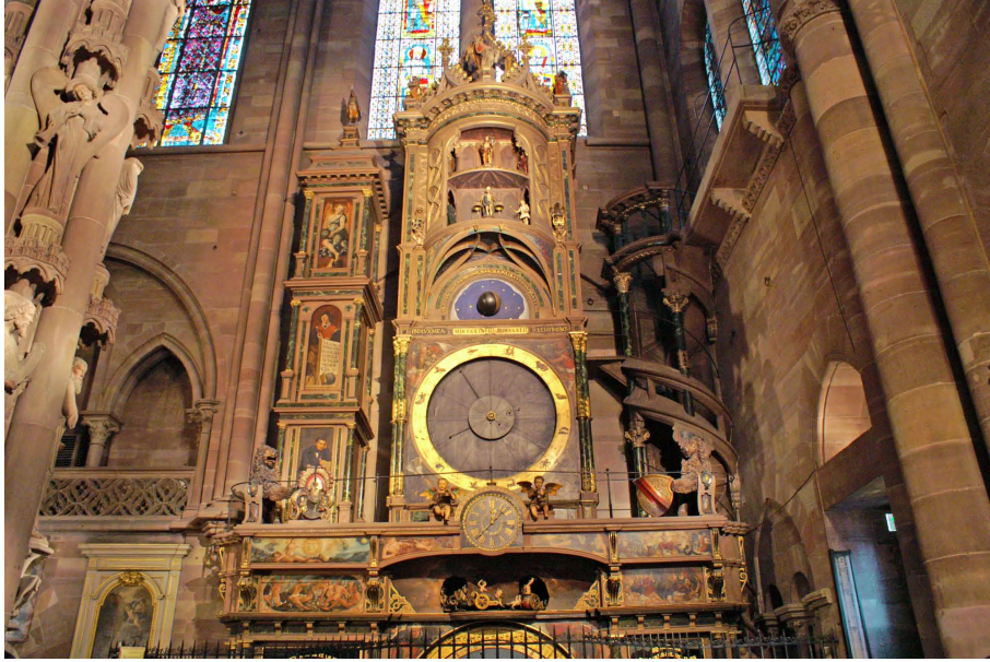
Figure 1: An example of classical analog simulator: the astronomical clock of Notre Dame de Strasbourg. Built in the fourteenth century, this device simulates the motion of planets in the solar system.
