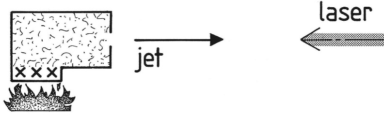
Figure 1.11: An atomic jet coming out from an oven through a small hole is slowed down by a counter-propagating resonant laser beam. Picture taken from [73].
