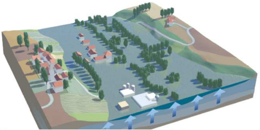
Figure 7: Illustration of the development of phreatic flooding. Reproduced from de Choudens, (2008).
