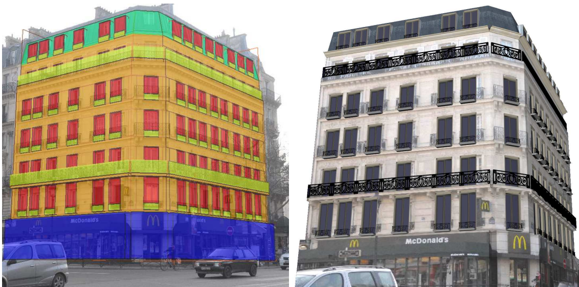
Figure 5.14: 3D reconstruction of a building with multiple facades visible from the street. Note that floors align seamlessly along the different facades.
