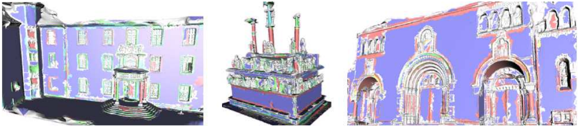
Figure 2.6: Reconstruction of different challenging scenes, based on the hybrid representation developed in [Lafarge 2010] (The following color code was used: purple=plane, pink=cylinder, blue=cone, yellow=sphere, green=torus, gray=mesh). Despite undeniable false positive and false negative cases with respect to the primitive detection, the results are quite promising. Image courtesy of [Lafarge 2010].
