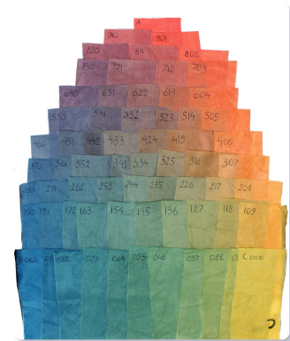
A.30 Real-Life Example of a Mayer's Triangle for Mixing Irgalan Dyes.
