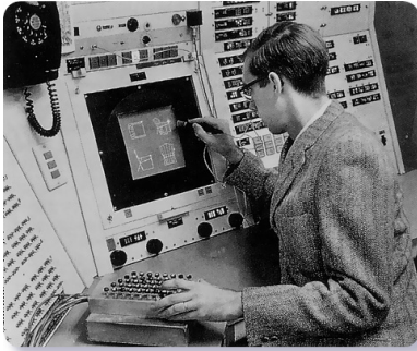
1.6 Ivan Sutherland's Sketchpad Console Controlled by a Light Pen and Command Button Box.
