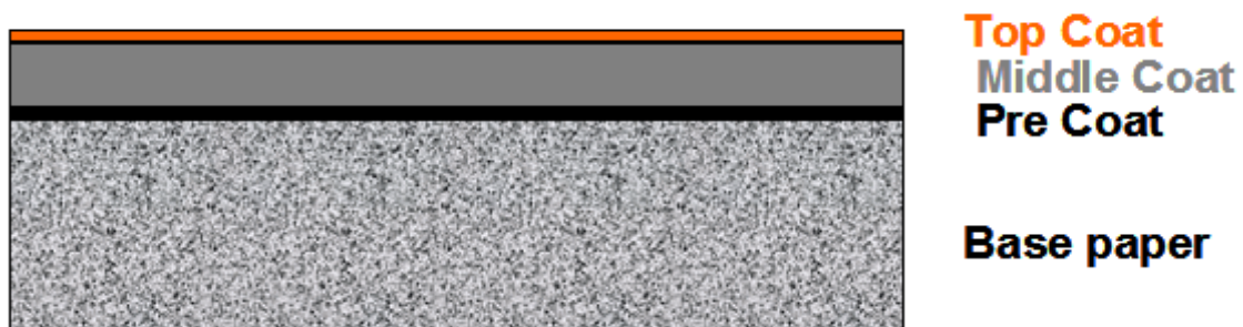
Figure 55: An example of the depth ratio used in curtain coating for WFC paper.
