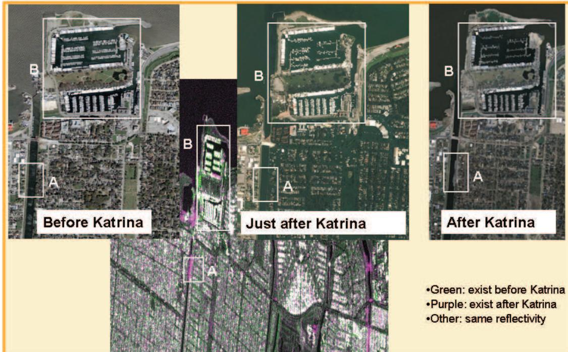
Figure 4.4.8: Change detection analysis by using the SAR reflectivity. Top) three aerial orthophotos taken over the same part of the city before, during and after the Katrina event to illustrate visually the changes due to the hurricane event. Bottom) RGB combination of the mean SAR reflectivity before and after the event, the same as in figure 4.4.7.
