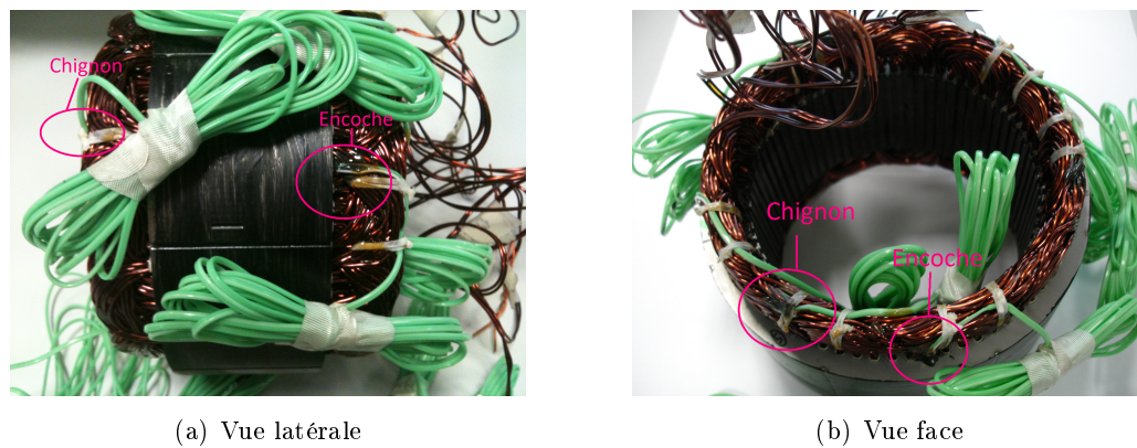
FIGURE IV.11 – Emplacement des thermocouples
