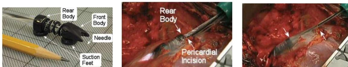
**Figure I.6 :** The HeartLander robot (source: [Riviere et al., 2006]).
