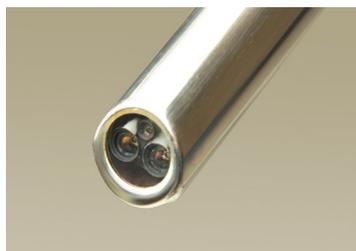
**Figure II.16** : An example of a stereo endoscope integrated into the DaVinci surgical platform. Photo courtesy of Intuitive Surgical, Inc., 2008.
