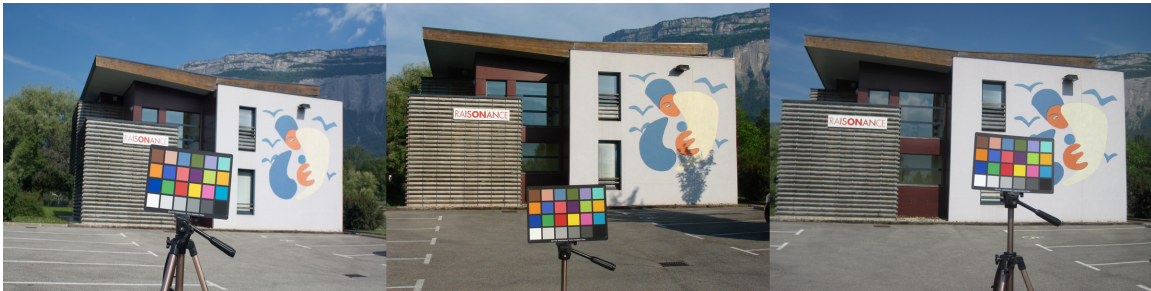
Figure 4.11: Example of images showing the ColorChecker in the scene during the acquisition.
