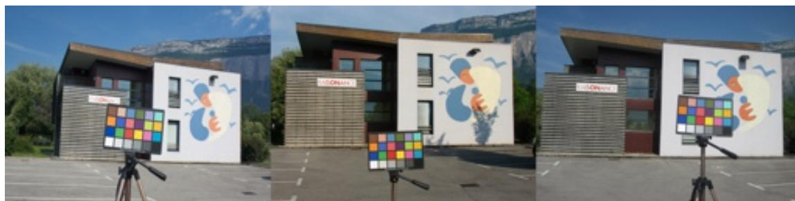
Figure 4.11: Example of images showing the ColorChecker in the scene during the acquisition.
