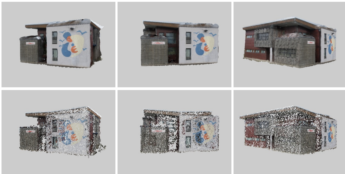
Figure 4.10: Example of the recovered 3D models: mesh and point cloud representations. Colors in both representations correspond to the mean value of pixels corresponding to the surface elements on the images where they are visible.
