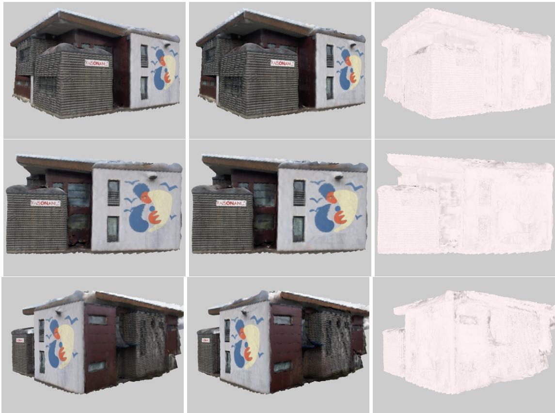
Figure 5.4: Albedo estimated for two subgroups of images of the first dataset. The first two columns show the estimated albedo and the third column presents the difference of the two estimations (darker zones correspond to large differences).
