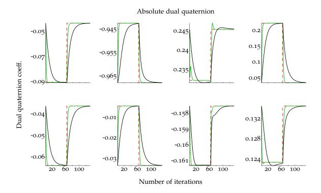
Figure 27: Coefficients of the absolute dual quaternion of example 3.4. The reference signal is represented by the *dashed red* curve, whereas the measured signals provided by the augmented Jacobian control law and the prioritized control law are represented by *solid green* and *solid black* curves, respectively.
