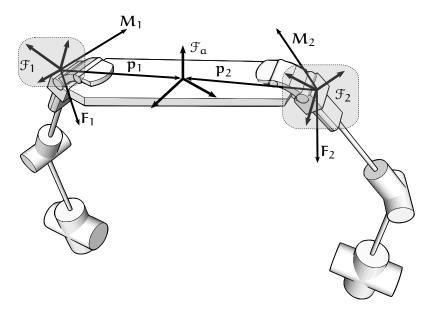
Figure 7: Two-arm manipulation using the symmetric control representation.  $\mathcal{F}_{\alpha}$  is a reference frame attached to the manipulated object,  $p_1$  and  $p_2$  are the virtual sticks, and  $F_i$  and  $M_i$  are force and moment acting at the i-th end-effector.
