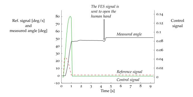
Figure 52: Time response for the successful trial shown in figure 51.
