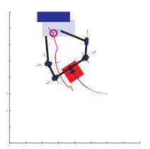
(e) The robot continues to perform the reactive behavior, following the person without the need of redefining the task. (f) The person stops and the robot arrives at the final spot, ready to pour the water.
