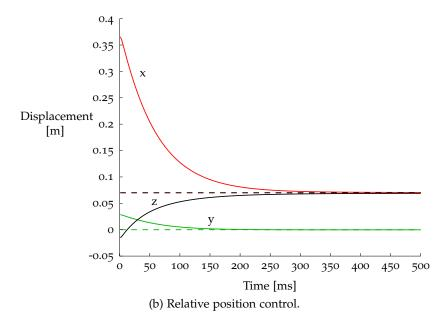
Figure 41: Water pouring: the robot reaches a predefined spot and simultaneously approaches one hand next to the other. The references are represented by *dash-dotted lines* and the responses by *solid lines*.
