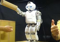
Figure 47: Teleoperation with collaboration: reaching the pipe (*left*) and handing it to another person (*right*).
