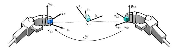
Figure 18: Cooperative dual task-space representation: the absolute and relative dual positions  $\underline{\mathbf{x}}_{\mathbf{q}}$  and  $\underline{\mathbf{x}}_{\mathbf{r}}$  completely describe the manipulation task.
