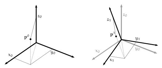
Figure 10: Frame rotation corresponding to the transformation  $p^1 = r_1^{0*} p^0 r_1^0$ .
