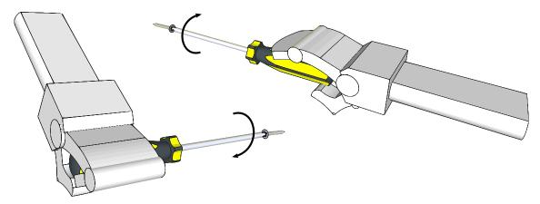
Figure 14: Robot hand manipulating a screwdriver: different hand poses, but the same description for the movement (i.e., from the point of view of the screw, the screwdriver must be rotated clockwise).
