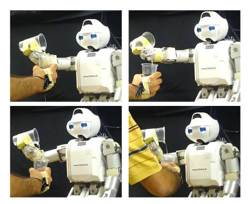
Figure 46: Task of pouring water.
