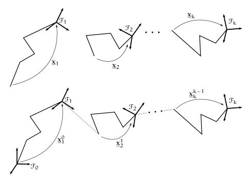
Figure 38: In the *top figure*, each kinematic subsystem is described by an intermediate rigid motion. When these subsystems are serially coupled (*bottom*), the rigid motion of one kinematic subsystem is given with respect to the previous one in the chain.
