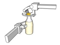
Figure 32: Opening a bottle. Not only the relative position should be controlled, but also the absolute orientation to avoid spilling the bottle's contents.
