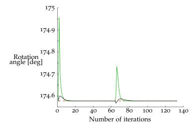
Figure 28: Angle between the robotic hands in the task of manipulating a broom (see example 3.4). The reference signal is represented by the *dashed-red* curve, whereas the measured signals provided by the augmented Jacobian control law and the prioritized control law are represented by *solid green* and *solid black* curves, respectivelly.
