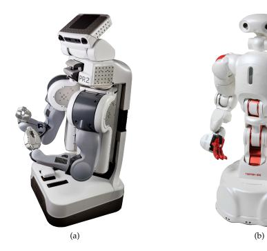
Figure 3: Two-arm mobile manipulators: (a) PR2 (Courtesy of Willow Garage); (b) Twendy-one (Courtesy of Sugano Laboratory, WASEDA University).
