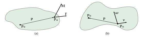
Figure 20: Wrenches and twists represented by dual quaternions: (*a*) in the wrench, the primary part corresponds to the force, whereas the dual part corresponds to the moment; (*b*) in the twist, the primary part corresponds to the linear velocity, whereas the dual part corresponds to the angular velocity.
