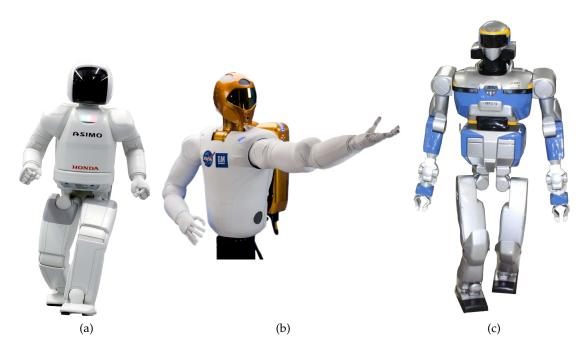
Figure 2: Humanoid robots which can potentially work side-by-side with humans: (a) ASIMO (courtesy of Honda), (b) Robonaut 2 (courtesy of NASA), and (c) HRP-2 (courtesy of AIST-CNRS).
