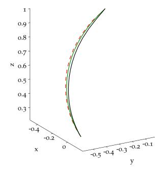
Figure 24: Trajectory executed by the KUKA arm of example 3.2. The dashed red, solid green, and solid black curves correspond to gains  $\lambda=0.01$ ,  $\lambda=0.05$ , and  $\lambda=0.1$ , respectively.
