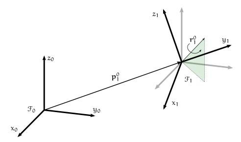
Figure 12: A rigid motion represented by quaternions: first a translation  $\mathbf{p}_1^0$  is performed, followed by a rotation  $\mathbf{r}_1^0$ .
