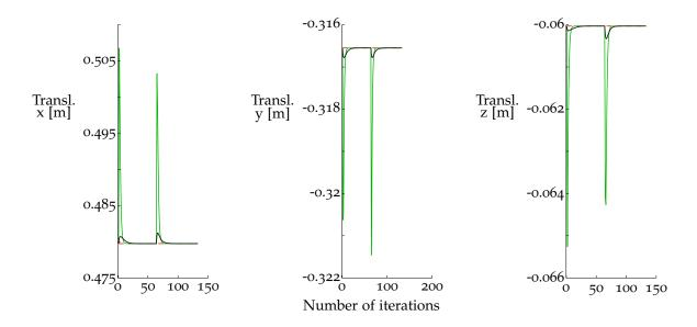
Figure 29: Relative translation between the robotic hands in the task of manipulating a broom (see example 3.4). The reference signal is represented by the *dashed red* curve, whereas the measured signals provided by the augmented Jacobian control law and the prioritized control law are represented by *solid green* and *solid black* curves, respectively.
