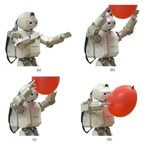
Figure 36: Grabbing a balloon. (a) Initial configuration. (b) Full dual position control: rough reaching phase. (c) Relative distance control. (d) Full dual position control: final configuration.
