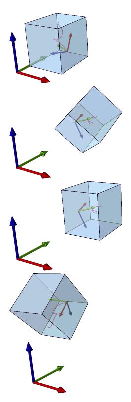
Initial pose. Note that before applying the decompositional multiplication, the box is always aligned with the base frame.
