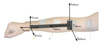
Figure 45: The human arm modeled as a one-link serial robot.
