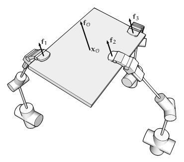
Figure 5: Augmented object model: the forces and moments  $f_i$  at the i-th end-effector are aligned with the operational force  $f_0$ . Using only this model, the internal forces cannot be controlled.
