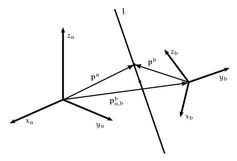
Figure 57: Plücker line with respect to frames  $\mathfrak{F}_{\mathfrak{a}}$  and  $\mathfrak{F}_{\mathfrak{b}}.$
