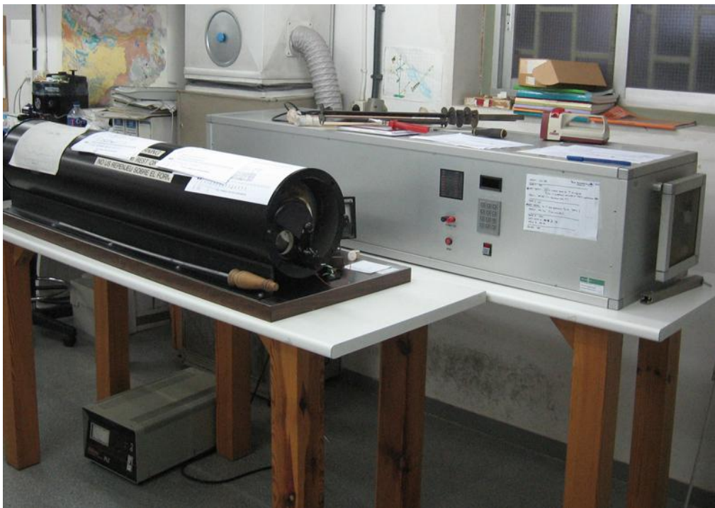
Annex I- 7: Thermal demagnetizer (Institute of Earth Sciences Jaume Almera, CSIC).
