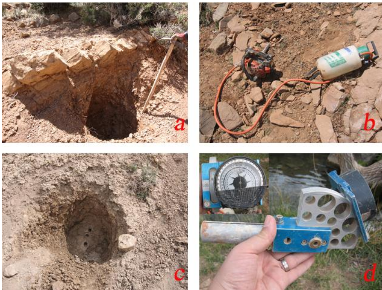
Annex I- 4: a,c) Delving for fresh sample point drill; b) portable gasoline-powered drill; d) compass for determining azimuth (Zagros-Iran field; 2008).
