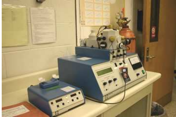
Figure 2.10: A high resolution ion beam coater system like the one used in Caen. The two sputtering ion sources are the yellow cylinders at the sides of the deposition chamber, while the etching gun is the one on top.
