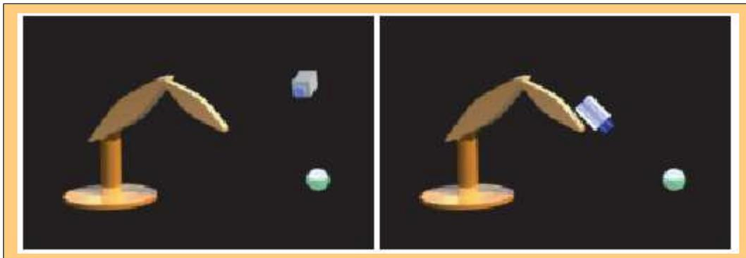
Fig. 2.8: (A gauche) Configuration eye-to-hand. (A droite) Configuration eye-in-hand.
