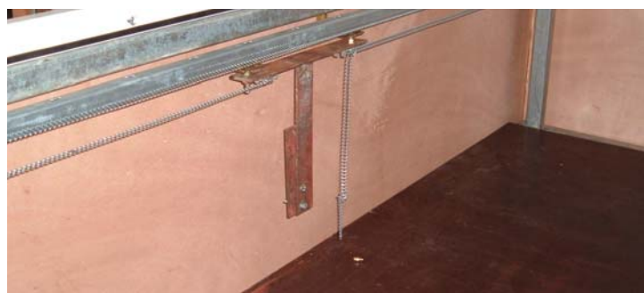
Figure II.13: le dispositif de translation
