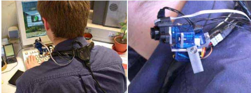
FIGURE 2.2. Active camera position to gesture recognition proposed by de Campos et al., (2006).
