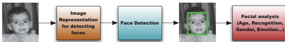
Figure 2.1: Automatic face verification system
