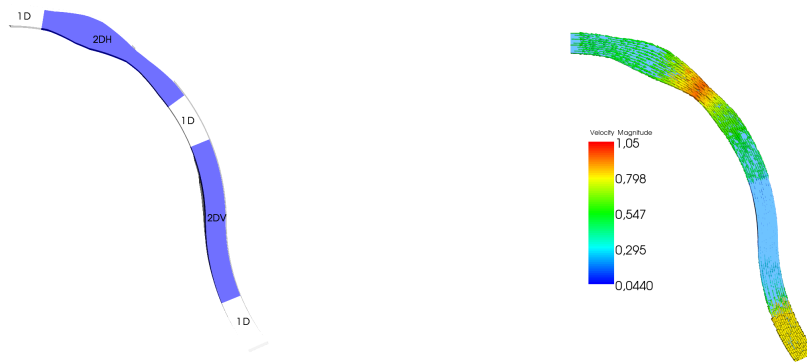
FIGURE 2.2.10. Definition of 2D regions and top view of velocity after coupling
