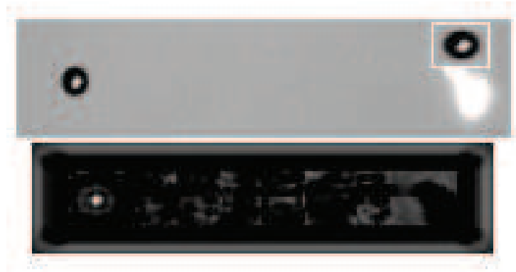
Figure 4.3: Images of a correlation method applied to track a glass spherical bead. The bottom image is the result of the correlation method applied to the top image. In the top right corner the template is shown.
