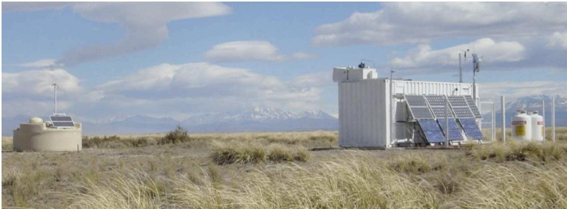
Figure 4.13: The Central Laser Facility, including the container, the solar panels and the propane heater, and the nearest SD tank, called Celeste. The tank, linked to the CLF by a fibre, receives laser light when a shutter, mounted on the optical table, is opened. The procedure allows synchronizing the SD array and the FD telescopes.
