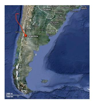
Figure 6.1: **Example of a back trajectory from the Malargüe location, from HYSPLIT.** The initial height is fixed at 500 m above ground level.
