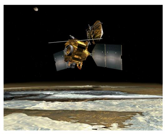
The Compact Reconnaissance Imaging Spectrometer for Mars aboard the Mars Reconnaissance Orbiter is devised to study water occurring as polar ice, as clouds and vapor in the atmosphere, locked in minerals, and as ice or groundwater below the surface. Credit: NASA/JPL-Caltech.
