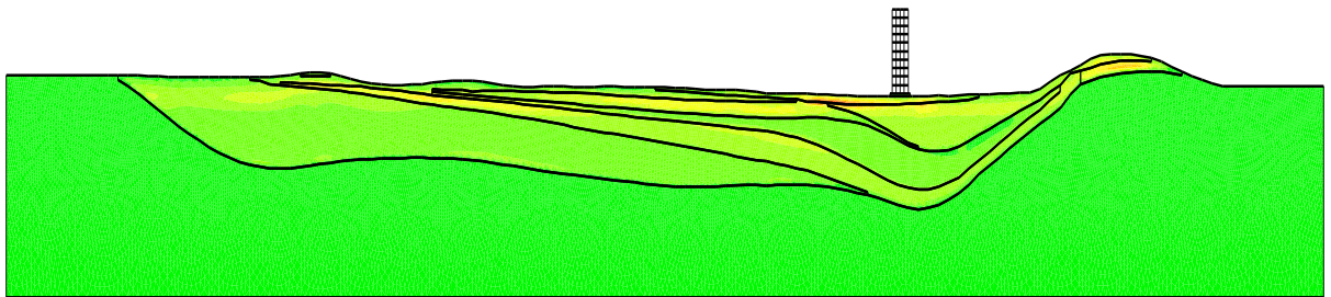
Figure 6.25: Maximum shear strain for 0.1g outcropping PGA in Nice basin
