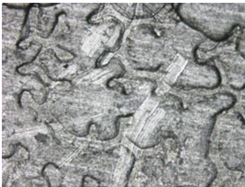
Figure 4.8 Optical microscopy image of steel surface(200 \mu m) after wedge test (PU2)
