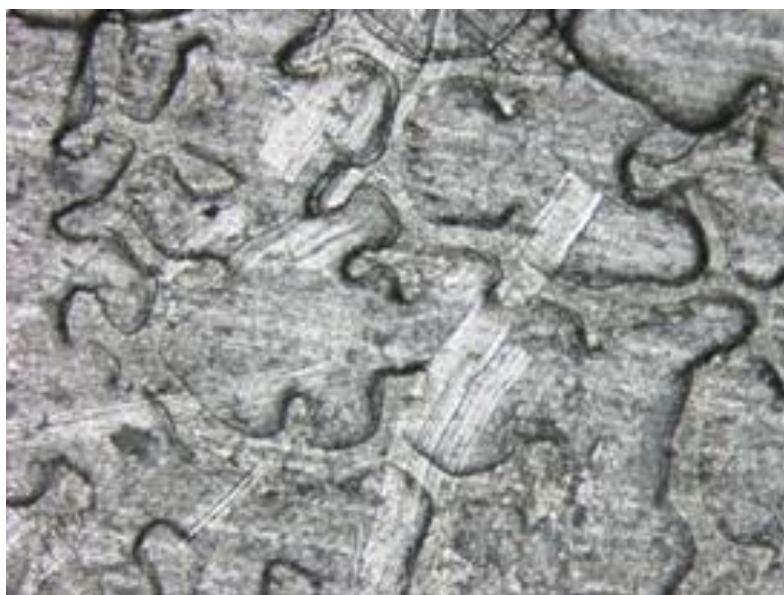
Figure 4.8 Optical microscopy image of steel surface(200µm) after wedge test (PU2)
