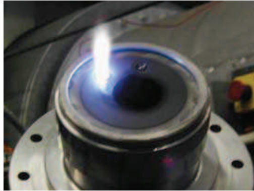
Figure 1.19. Plasma Igniter in operation (Matveev et al. , 2009)
