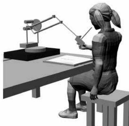
**Fig. 1. Global and schematic view of the Telemaque working station.** Children were seated in front of a table upon which the letters generated by the visuo-haptic interface were displayed on a horizontal computer screen. Children had to hold a pen attached to force-feedback arm controlled by the Telemaque software.
