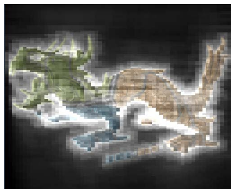
Figure 6.14. Display of ray execution times in grayscales for a 1024^3 voxels scene and 16^3 bricks. Time is measured per tile corresponding to the SIMD execution entities (warps) of the GPU.
