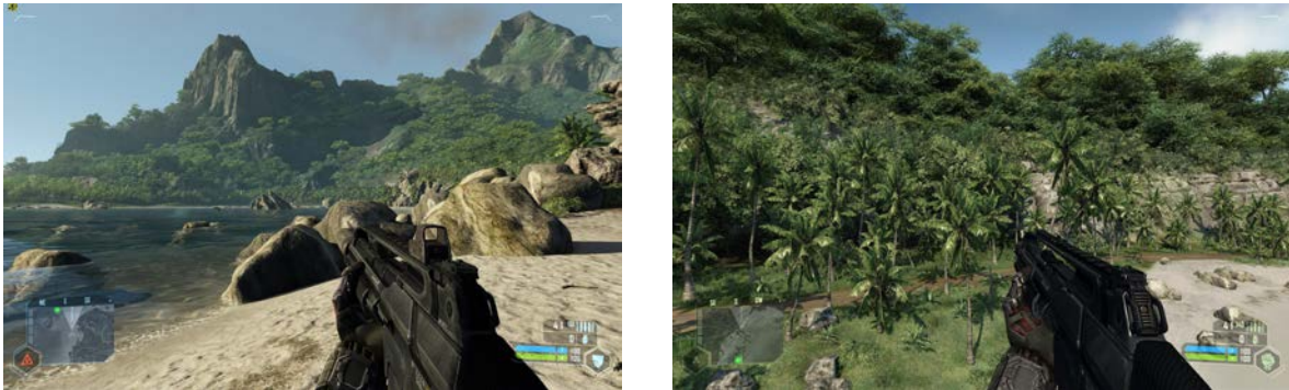
Figure 1.8. Illustration of forest rendering in video-game. Trees are rendered using multiple representations, usually high resolution geometry for closeup views, simplified geometry for medium distance, and impostors for far views. Such a scheme induces low quality geometry filtering and popping artifacts. Source: Crysis (Crytek)
