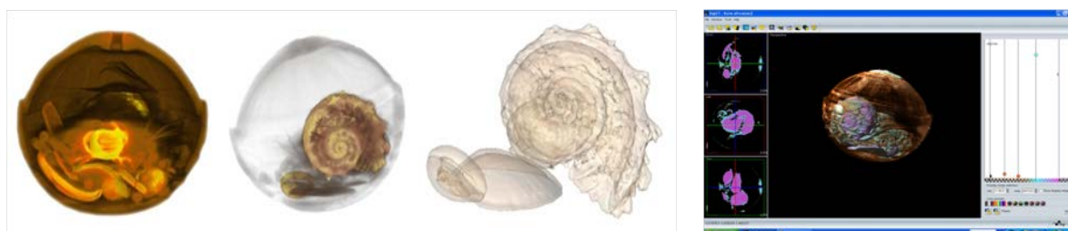
Figure 1.18. Examples of the visualization of archaeological objects scanned using X-Rays and reconstructed using tomography. Source: Digisens 2009
