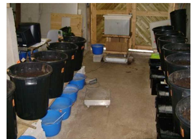
Figure 14. Large scale vermifilter and mesocosm experiment in a not insulated building; both received the same liquid added each day
