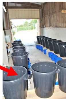
Figure 14. Large scale vermifilter and mesocosm experiment in a not insulated building; both received the same liquid added each day
