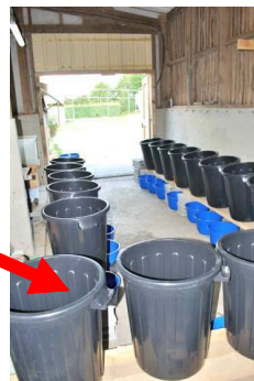
Figure 27. Large scale vermifilter and not insulated building for mesocosm experiment; both received the same liquid added each day
