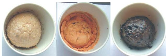
**Fig. 1** Photos of catalyst **3** Ce<sub>0.95</sub>Cr<sub>0.05</sub>O<sub>2</sub>, **17** Ce<sub>0.96</sub>Zr<sub>0.02</sub>Fe<sub>0.02</sub>O<sub>2</sub> and **14** Ce<sub>0.92</sub>Cu<sub>0.08</sub>O<sub>2</sub>, before impregnation with the active metals, showing the homogeneous mixing of the dopants and the ceria. In the case of copper (**14**), the black colour indicates the presence of CuO instead of Cu<sub>2</sub>O, which is typically yellow/red.<sup>43</sup>
