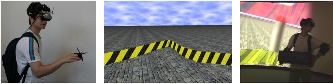
Figure 6.1 – The Magic Barrier Tape displays the boundaries of the real workspace as a virtual barrier tape, and uses a hybrid position/rate control to travel in the VE. The user (left) “pushes” on the Magic Barrier Tape (center) to move inside the VE when he reaches the workspace boundaries. Any tracked body part can be used to trigger the Magic Barrier Tape (right).
