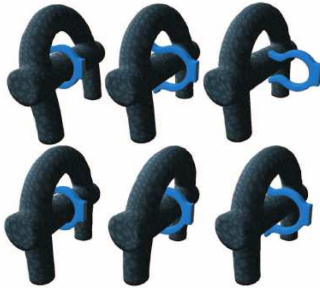
Figure 1.16 – Linear deformations using an LCP formulation: snap-in (top) and snap-out (bottom) tasks on deformable pipes with deformable proxies and friction feedback [5].
