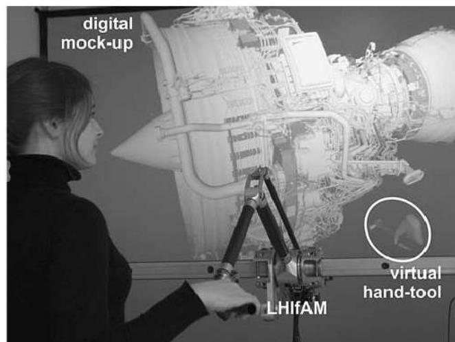
Figure 1.25 – High-level multimodal integration for virtual prototyping: a distributed approach with visual, acoustic and kinesthetic feedback [122].
