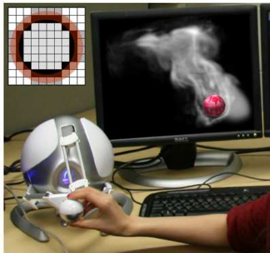
Figure 1.23 – Physically based haptic interaction with smoke. Visual rendering of the application with a proxy discretization into the Eulerian grid (top left) [26].
