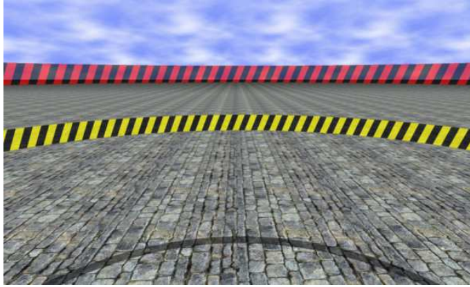
Figure 6.2 – The three Magic Barrier Tape visual cues to show the workspace boundaries: the main virtual barrier tape (middle), the warning tape (top) and the tapes shadow (bottom).
