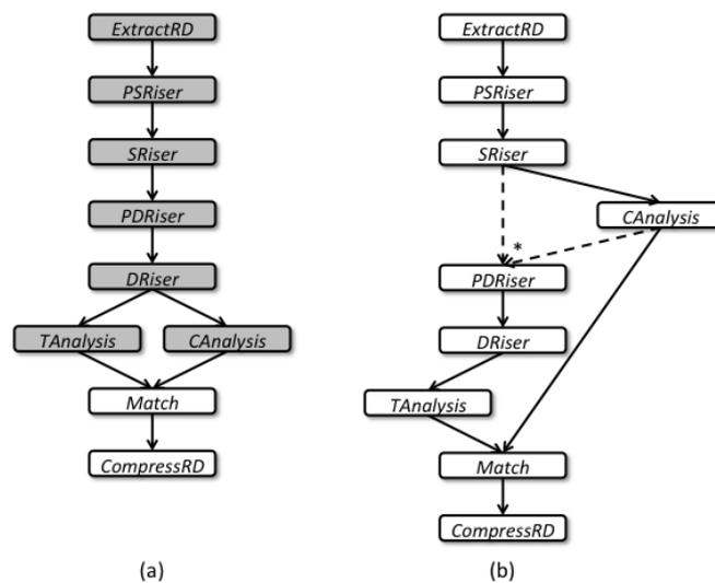
Figura 54 - Workflow RFA (a); Workflow RFA otimizado (b)
