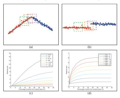
Figure 3.4: z-variance of the plane estimation depending on the percentage of points from another model. (a) First experiment: two intersecting planes forming an angle  $\alpha$  with their orientations. (b) Second experiment: two horizontal planes separated by a step along the z-axis. (c) Results of first experiment for different angles. (d) Results of second experiment for different steps.
