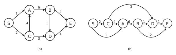
Figure 5.8: (a) A DAG  $\mathcal{G}(\mathcal{V}, \mathcal{E})$  and (b) its linearization.
