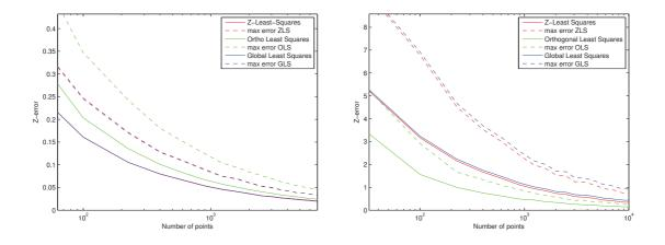
Figure A.2: Mean error (plain lines) and max error (dashed lines) along the z-axis. In red, least squares with  $c = cste \neq 0$ ; in green, orthogonal least squares; in blue, least squares with  $||\mu||_2^2 = 1$ . Left image: Data set corrupted with an additive Gaussian noise on the z-axis only. Right image: Data set corrupted with an additive Gaussian noise on each axis.
