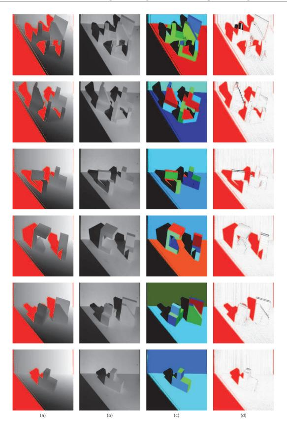
Figure 4.3: Experiments on range images. (a) Range values (red parts are unknown). (b) Intensity image. (c) Classification obtained with our algorithm. (d) Reprojection error (the larger the error, the darker the image)
