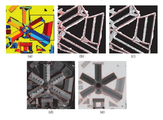
Figure 5.7: Results of the *a contrario* criterion on Toulouse dataset. (a) Input planar classification. (b) and (c) Binary re-projection error and found contours before (b) and after (c) NFA filtering. (d) Reference image and NFA validated contours. (e) Ground truth disparity map and validated contours. One can see that the validated contours tend to fit the data.
