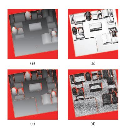
Figure 4.9: Interpolation of the missing points in disparity map obtained with Sabater's algorithm. (a) Interpolated disparity map by reprojection from our classification. (b) Error between the interpolation and the ground truth (the larger the error, the darker the image). (c) Interpolated disparity map with median filtering. (d) Error between the interpolation and the ground truth.
