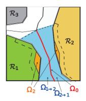
Figure 5.2: Construction of a search region.  $\mathcal{R}_1$  and  $\mathcal{R}_2$  are the two regions for which we want to refine the separation. The search region  $\mathbb{R}_{1,2}$  is defined as the dilatation by a correlation window of  $\Omega_0$  (edge of the two Voronoi cells, in red here),  $\Omega_1$  (unknown points, in blue) and  $\Omega_2$  (points possibly belonging to both planes, in orange). The dilatation is delimited by the dash lines.
