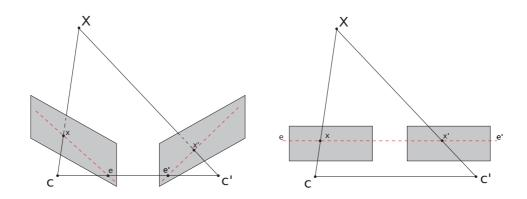
Figure 1.1: Epipolar rectification. Left: camera configuration before rectification. Right: rectified cameras. The 3D point **X** and the two camera centers C and C' define a plane. Its intersection with the two image planes defines two lines: the epipolar lines for **X** (dashed red lines). The intersection of the epipolar lines of **X** with the *baseline* (CC') (*e* and *e'*) are called the epipoles. They represent the projection of the camera centers onto the other image plane.
