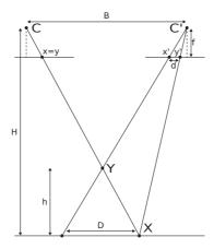
Figure 1.2: Computation of the depth of a 3D point in epipolar geometry. From Thales theorem, one can see that the height h of Y is proportional to the shift in position d.
