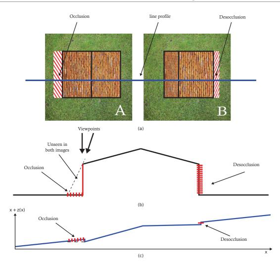
Figure 5.5: Occlusion in stereo-vision. (a) Two views of a same scene. (b) Disparity values along the blue line. (c) x + z(x).
