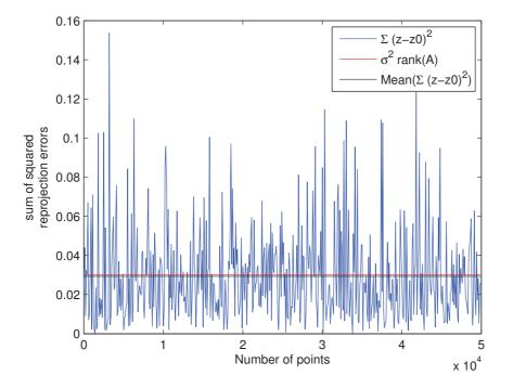
Figure A.1: Sum of squared re-projection errors for simulated data. The figure shows that this sum do not depend on the number of points. Moreover, the mean result is close to what is expected from Proposition 4.
