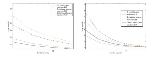
Figure A.3: Mean error angle (plain lines) and max error angle (dashed lines) between the real plane and the estimated plane. In red, least squares with  $c = cste \neq 0$ ; in green, orthogonal least squares; in blue, least squares with  $||\mu||_2^2 = 1$ . Left image: Data set corrupted with an additive Gaussian noise on the z-axis only. Right image: Data set corrupted with an additive Gaussian noise on each axis.
