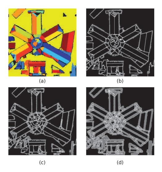
Figure 5.3: Example of construction of the search on Toulouse dataset. (a) Input classification. (b) Region formed using the points with unknown disparities. (c) Regions without intersection points. (d) Regions without adhesion points (dilatation of (b) and (c))
