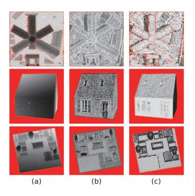
Figure 4.12: Disparity obtained with RAFA algorithm. From top to bottom: Toulouse, "Bergerie" and "Village". (a) Disparity map. (b) Precision estimated from Eq. 4.5. (c) Error to the ground truth.
