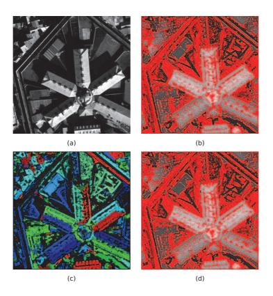
Figure 4.10: Toulouse PELICAN dataset. (a) Reference image. (b) Disparity map obtained with Sabater's algorithm. (c) Classification result with our algorithm. (d) Reprojection on the planes found with our classification
