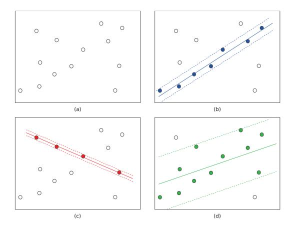
Figure 2.1: Influence of the distance threshold parameter on plane computation. (a) Initial point set. (b) Optimal detection threshold. (c) Too small threshold. (d) Too large threshold. A wrong threshold may change a lot the value of the computed plane.
