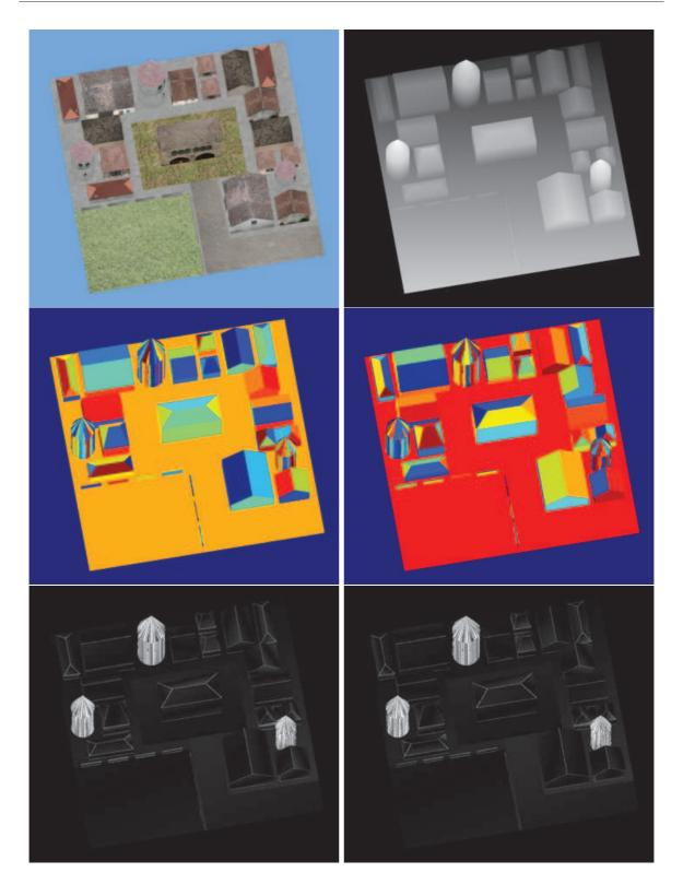
Figure A.4: Results on Village1 disparity map. First line: reference image(left) and disparity map(right). Second line: plane classification obtained with least squares minimization with c = cste(left) and orthogonal constraint(right). Third line: residual error obtained with least squares minimization with c = cste(left) and orthogonal constraint(right).
