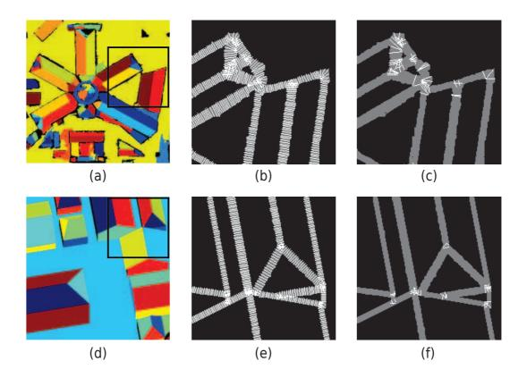
Figure 5.13: Example of search region partitioning. First raw Toulouse dataset. Second raw Village dataset. (a) and (d) input classification. (b) and (e) Result of the search region partitioning as explained in Section 5.5.2. (c) and (f) simplification of the partition.
