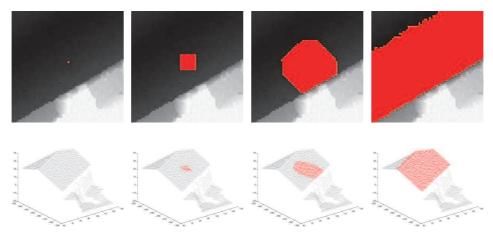
Figure 3.2: Region growing. From an initial point, the points are added progressively if the distance between the real disparity and the projection on the estimated plane is less than a threshold  $\tau_z$ . Top row: disparity map. Bottom row: corresponding 3D points.
