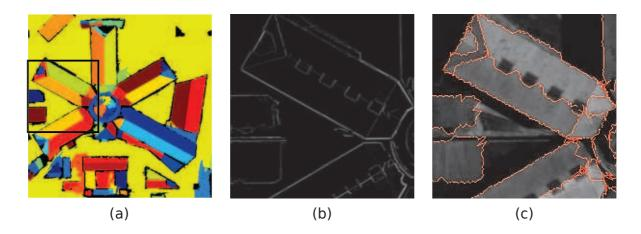
Figure 5.4: Resulting contours between planes using the gradient energy. (a) Input disparity map classification. (b) Zoom of the gradient of the reference image into the search regions. (c) Resulting contours. This energy seems very adapted in cases where the 3D separation corresponds to a unique highly contrasted curve, but, however fails in cases where the gradient is not very contrasted or where the most contrasted curve is not the right one.
