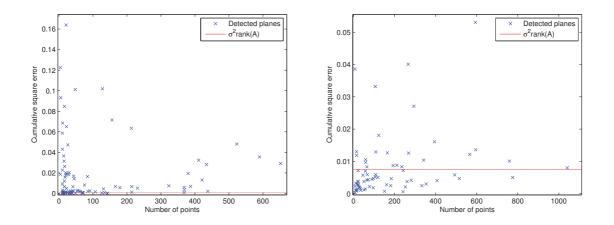
Figure 3.7: Cumulative square re-projection error for each plane detected:  $\sum_{\mathbf{x}\in G} (z(\mathbf{x}) - z_{\pi}(\mathbf{x}))^2$ . (a) Toulouse ground truth. (b) Village 1 ground truth.
