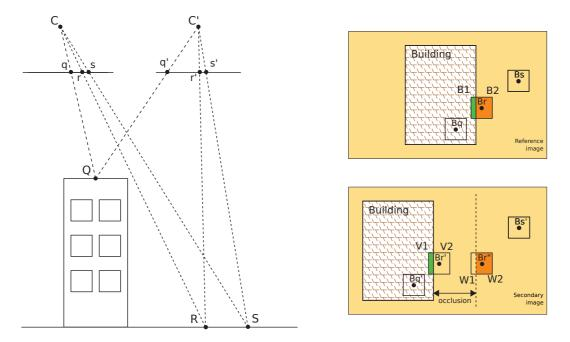
Figure 1.3: Adhesion artifact. The correct disparity to  $\mathbf{r}$  is  $\mathbf{r}$ " but  $B_r$  is mismatched to  $B_{r'}$ . This figure was inspired from a figure on adhesion in Neus Sabater's PhD's manuscript [Sabater, 2009].
