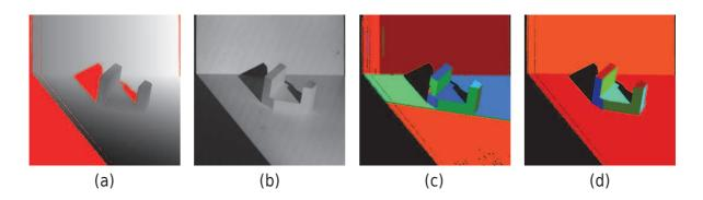
Figure 4.2: (a) Input range image (red parts are missing points). (b) Intensity image. (c) Classification with the original algorithm of Chapter 3. (d) Classification after correction of our algorithm.
