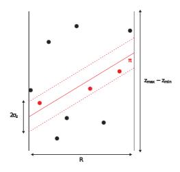
Figure 2.3: Probability of a random point to be associated to plane  $\pi$
