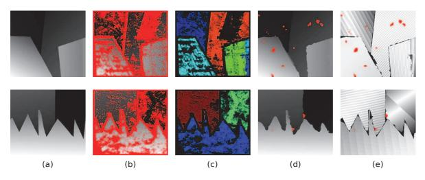
Figure 4.11: "Venus" and "Sawtooth" disparity maps. (a) Ground truth disparity map. (b) Disparity maps obtained with Sabater's algorithm. (c) Classification obtained with our algorithm. (d) Interpolated disparity map from our classification. (e) Error between interpolation and ground truth (the darker the image, the larger the error).
