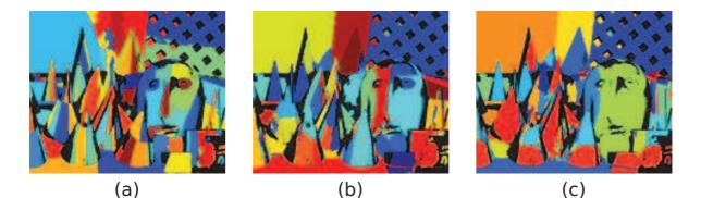
Figure 2.6: Classification obtained with different precisions. (a) precision=1 pixel, 85 planes detected; (b) precision=2 pixels, 44 planes detected; (c) precision=5 pixels, 23 planes detected.
