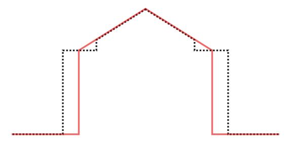
Figure 1.4: Continuous line: cut of a depth map of a house. Dotted line: estimated depth affected by adhesion. Adhesion causes the dilatation of the depth value of the roof edges.
