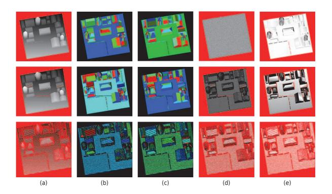
Figure 4.8: Result on the "Village" dataset. From top to bottom: ground truth + additive Gaussian noise, MicMac algorithm, Sabater's algorithm. (a) Disparity map (red parts are missing points). (b) Classification with the initial algorithm. (c) Classification after the correction. (d) Initial error to ground truth (dynamique: 0 pixel = white 0.1 pixels = black). (e) Final error after reprojection on the classification planes (dynamique: 0 pixel = white 0.1 pixels = black).
