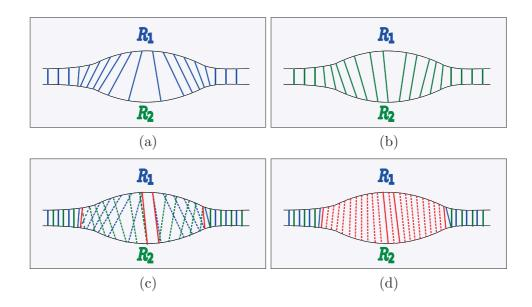
Figure 5.10: Division into subregions. (a) Find for each point in  $\partial \mathcal{R}_1$  its closest point in  $\partial \mathcal{R}_2$ . (b) Find for each point in  $\partial \mathcal{R}_2$  its closest point in  $\partial \mathcal{R}_1$ .(c) Remove the intersecting segments. In this case this happened because the search region was enlarged. (d) Interpolate the missing segments.
