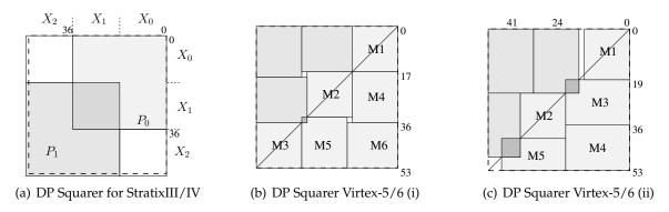
Figure 6.10 Double-precision squaring. Tilings for StratixIII/IV and Virtex-5/6 devices
