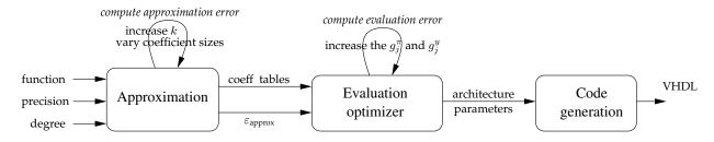
Figure 7.2 Automated implementation flow
