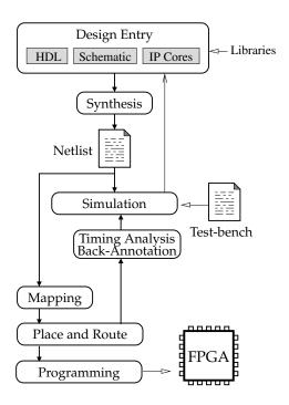
Figure 2.8 Classical FPGA design flow
