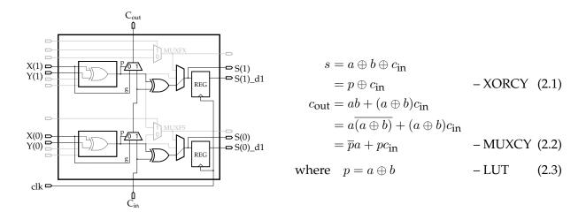
Figure 2.3 Ripple-Carry Adder (RCA) implementation in Virtex-4 devices
