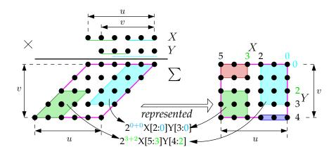
**Figure 6.1**  $u \times v$ -bit multiplier
