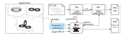
**Figure 11.1** Automation flow: the C code is first parsed by the Bee research compiler; FloPoCo is then invoked for generating the required arithmetic pipeline; the pipeline information is then passed back to the Bee compiler for use in operation scheduling; next, the pipeline depth adjustments are sent to FloPoCo for generating the final VHDL.
