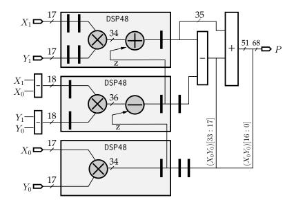
Figure 6.3 34x34bit multiplier using Virtex-4 DSP48
