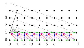
**Figure 11.9** Inter tile slice iteration domain for Jacobi 1D stencil code. The parallel hyperplane has  $\vec{\tau} = (1,3)$  and describes the tile-slices which can be executed in parallel. The dashed lines indicated various translations of the hyperplane  $H_{\vec{\tau}}$  showing different levels of parallelism.
