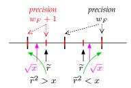
**Figure 8.1** Deducing the correctly rounded value of  $\sqrt{x}$  on  $w_F$  bits from a faithfully rounded result on  $w_{F+1}$  bits
