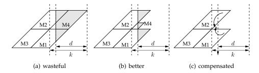
**Figure 6.12** Truncation applied to multipliers. Left: Classical truncation technique applied to DSPs. Center: Improved truncation technique; M4 is computed using logic. Right: FPGA optimized compensation technique; M4 is not computed.
