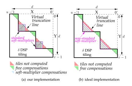
Figure 6.13 Tiling truncated multiplier using DSPs and soft-core multipliers
