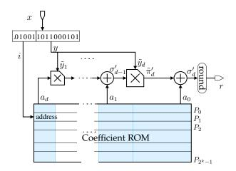
Figure 7.5 The function evaluation architecture
