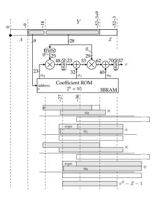
**Figure 9.5** The architecture evaluating  $e^Z - Z - 1$  for Virtex-5/Virtex-6
