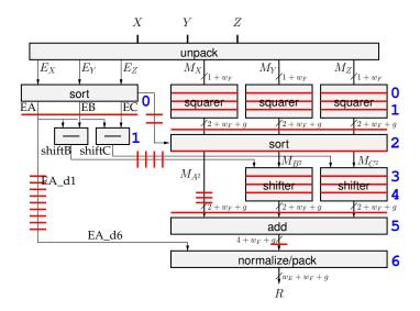
Figure 4.2 Optimized architecture for the Sum-of-Squares operator
