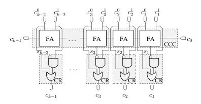
Figure 5.9 Carry Computation Circuit with Carry Recovery
