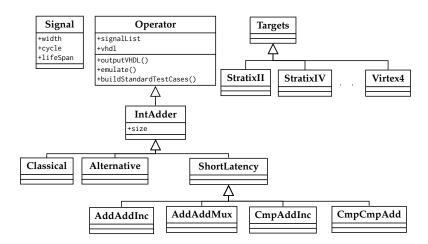
Figure 5.1 FloPoCo class structure for binary addition
