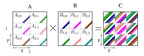
Figure 11.7 Matrix-matrix multiply using blocking
