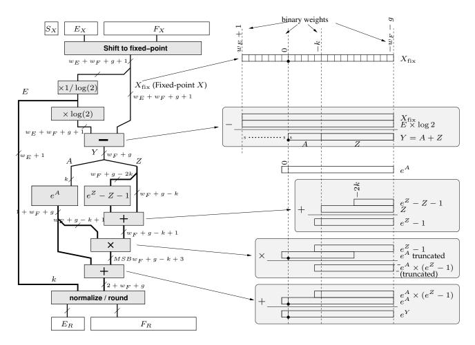
Figure 9.3 Architecture and fixed-point data alignment
