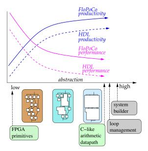
**Figure 4.1** Productivity in porting applications to FPGAs and the relative performance of these circuits provided the different levels of abstraction are provided for circuit description
