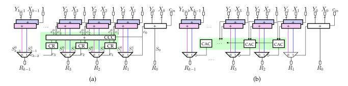
Figure 5.10 The AAM Carry-Select Architecture using (a) the CCC and CR and (b) the CAC
