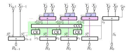
Figure 5.11 The CAI Carry-Increment Architecture
