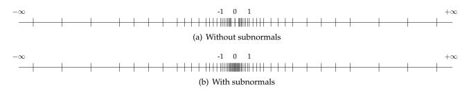
**Figure 3.1** Distribution of floating-point numbers in a system  $\xi(2,3,-2,3)$ , having a IEEE-754 equivalent p=3 and  $w_e=3$ . The -3 and 4 values of e are used to represent the special cases presented in table 3.2
