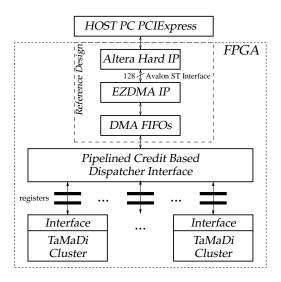
Figure 12.6 Global system architecture
