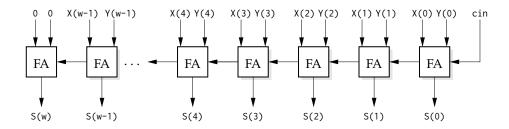
Figure 5.2 Ripple-Carry Adder implementation
