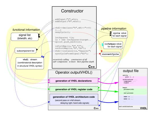
Figure 4.5 Simplified overview of VHDL generation flow
