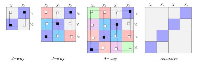
**Figure 6.2**  $u \times v$ -bit multiplier
