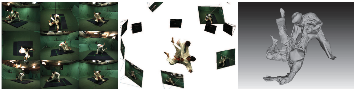
Figure I.1: Overview of multi-view shape from images: On the left: input images taken from the GRImage platform at Inria, that allows to acquire up to 32 synchronized and calibrated video data. On the middle we show the calibrated pictures in the 3D space at time t . On the right is an expected output: a tri-dimensional model representing the scene or object of interest obtained with [31].
