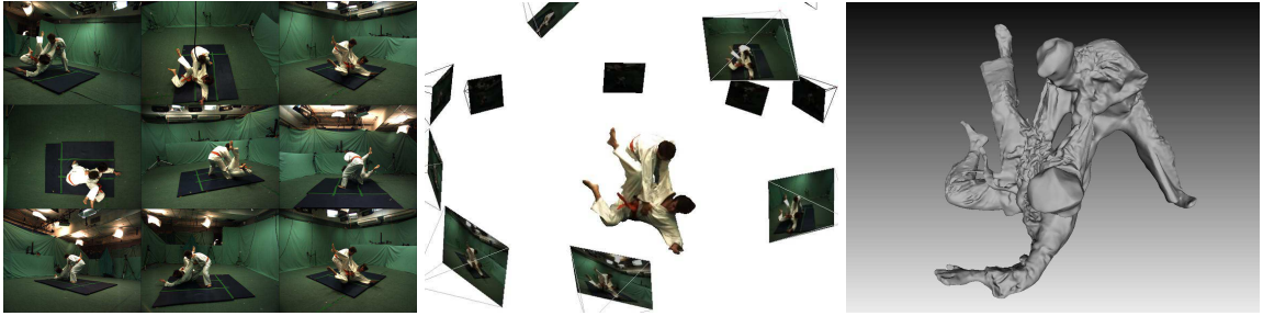
Figure I.1: Overview of multi-view shape from images: On the left: input images taken from the GRImage platform at Inria, that allows to acquire up to 32 synchronized and calibrated video data. On the middle we show the calibrated pictures in the 3D space at time t . On the right is an expected output: a tri-dimensional model representing the scene or object of interest obtained with [31].
