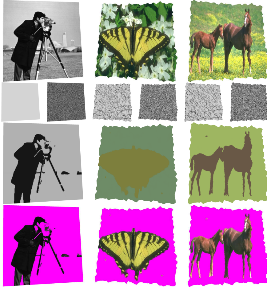
Figure IV.5: Segmentation results on meshes in the two-region segmentation on three different examples. From top to bottom: Input textured mesh; Mesh shape where the segmentation is performed and the initial random value of one component of \mathbf{Y} ; Recovered mean values of each region; Segmented object.
