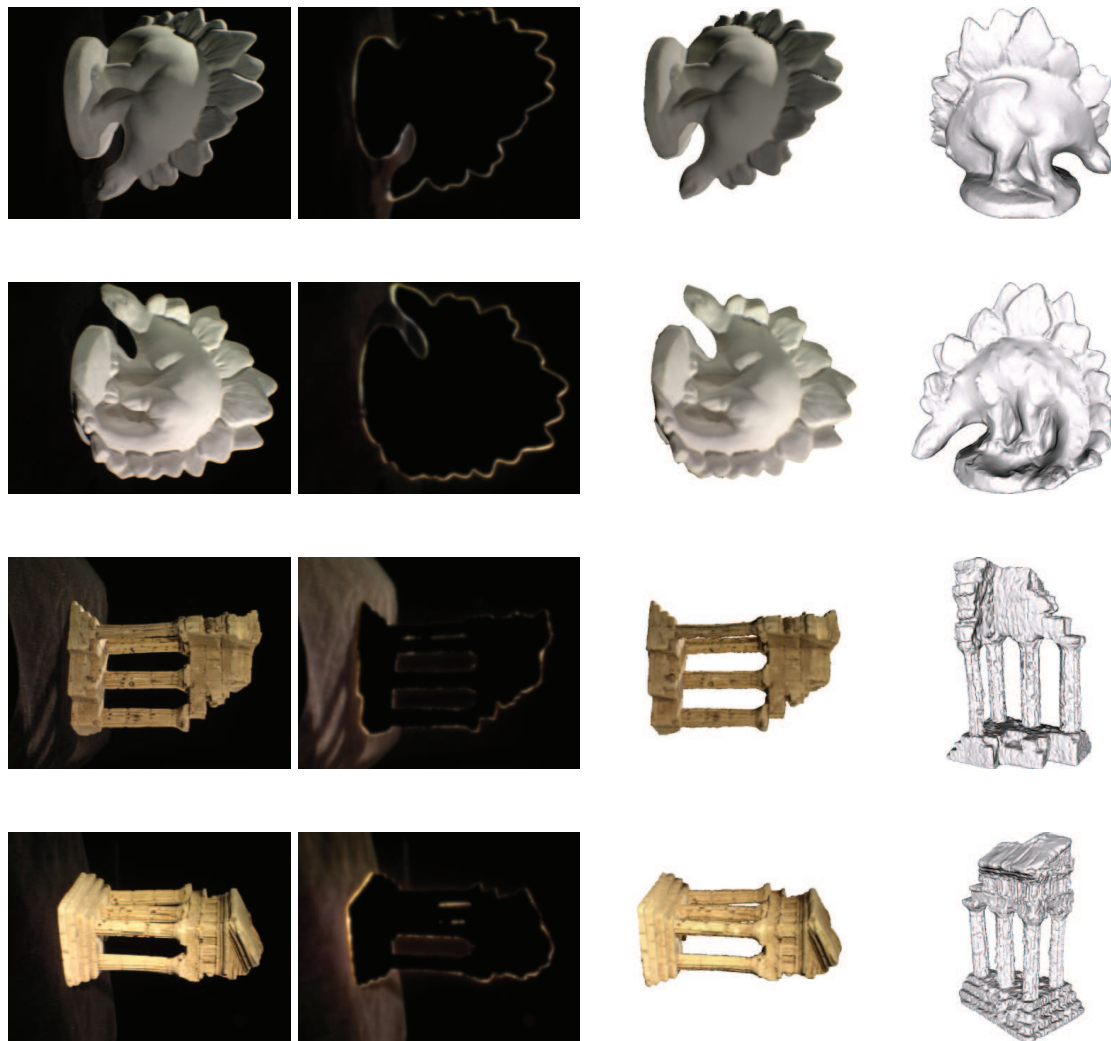
Figure III.3: Dino and Temple sequence (input data courtesy of [136]). From left to right: 1 of 16 input images; estimated background images (scaled by 2 for visualization); estimated radiance; estimated mesh seen from a different viewpoint.
