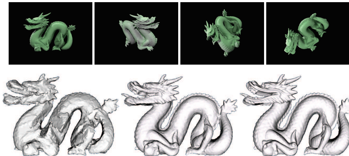
Figure III.2: Synthesized dragon sequence. Top row: 4 of 32 diffuse input images. Bottom row: Initial shape; recovered shape by our algorithm; ground truth model.
