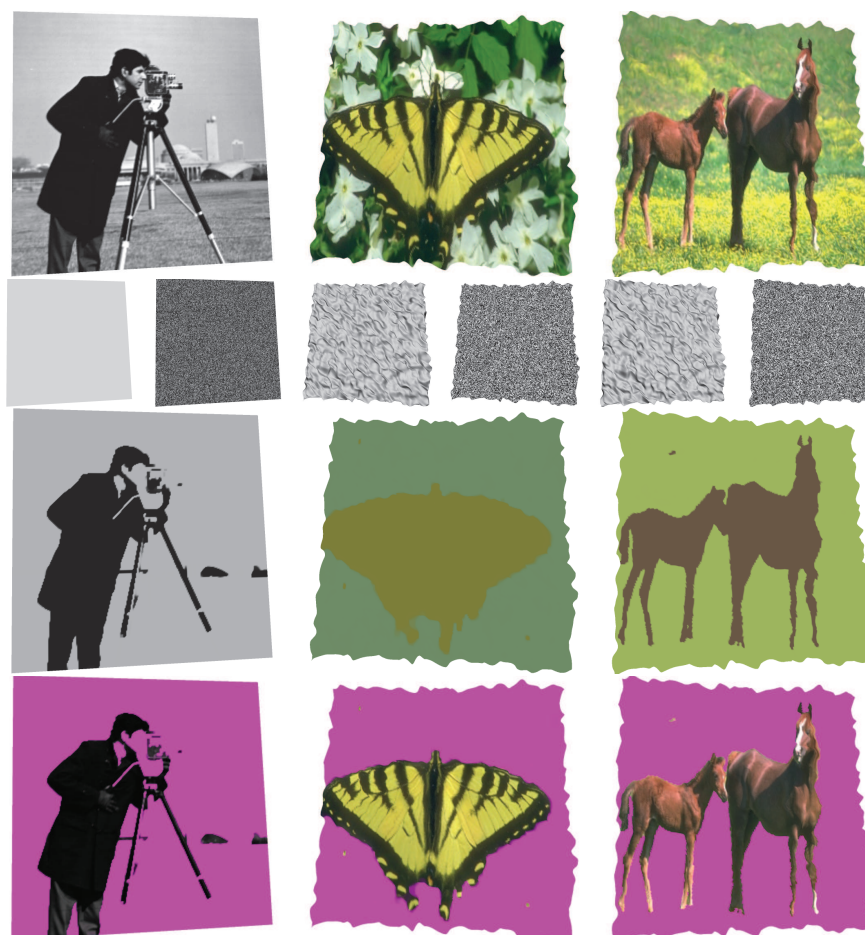
Figure IV.5: Segmentation results on meshes in the two-region segmentation on three different examples. From top to bottom: Input textured mesh; Mesh shape where the segmentation is performed and the initial random value of one component of Y ; Recovered mean values of each region; Segmented object.
