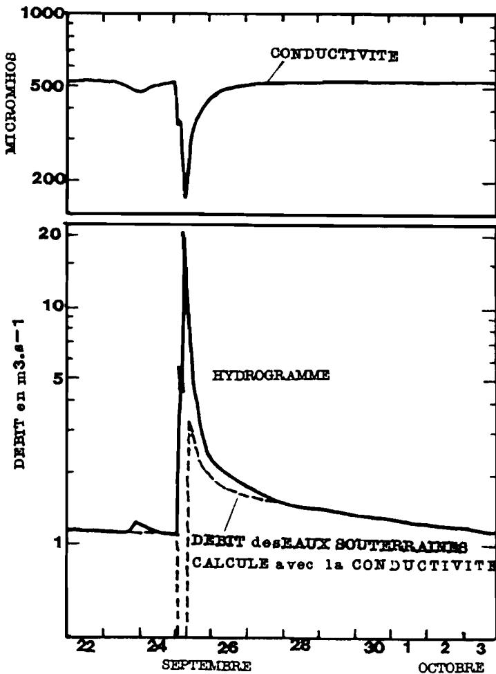
Fig. 110 : COURBES DE DEBIT, CONDUCTIVITE ET ECOULEMENT SOUTERRAIN CALCULE A FOUR MILE CREEK (TRACER, IOWA - SEP ET OCT 1963 - KUNKLE 1965)
