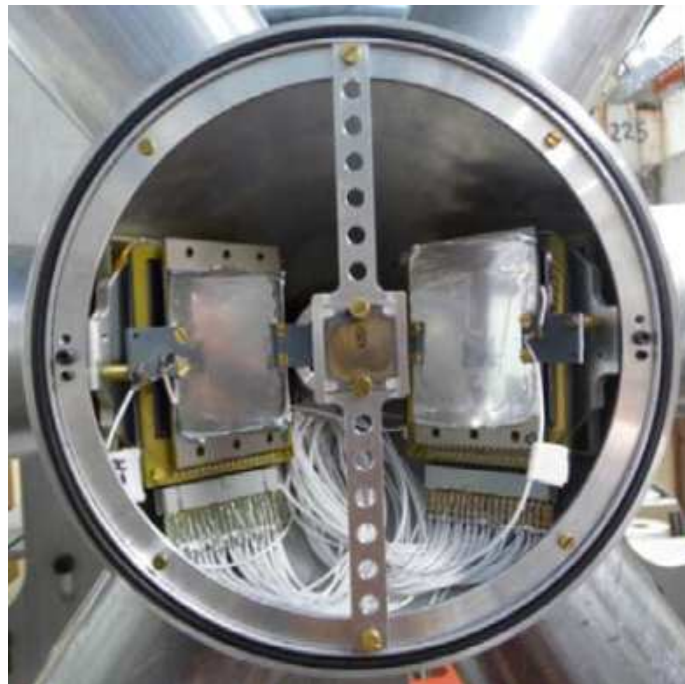
Figure 3.7: Front view of the reaction chamber. At the centre, one distinguishes the ^{174}\text{Yb} target surrounded by the two telescopes shielded with nickel frames and thin Mylar(Al) foils. The support for the telescopes and the reaction chamber have been designed and constructed at the CENBG.
